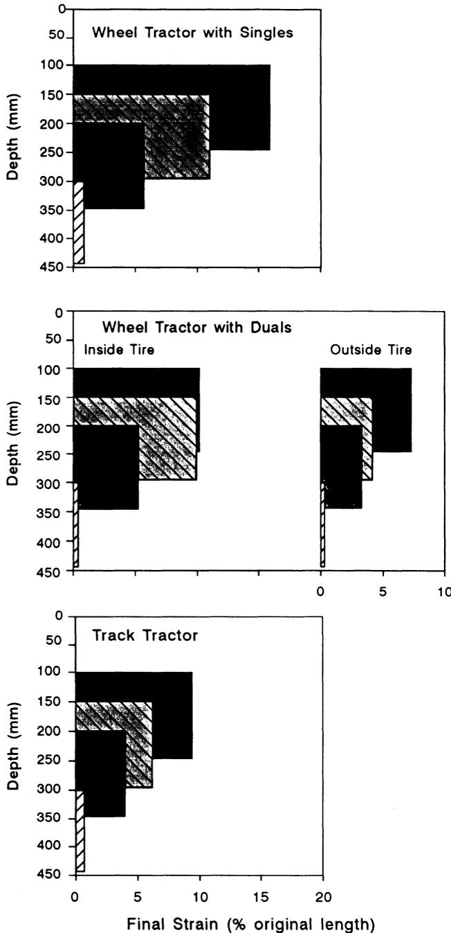
Figure 5—Average final strain with respect to depth for each tractor. Bar location represents initial location of transducer with respect to soil surface.
