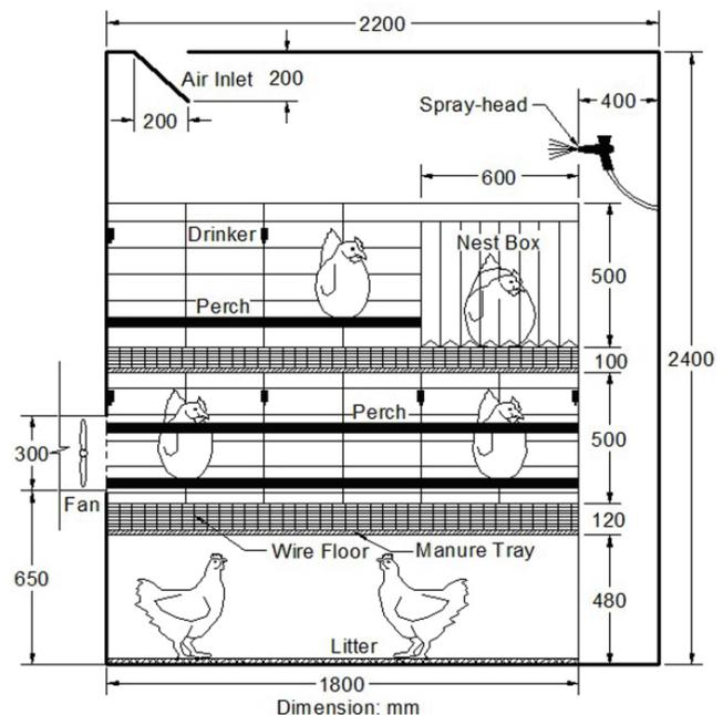
Figure 2. Longitudinal view of the aviary laying-hen chamber.
