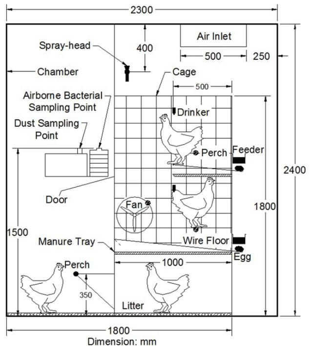
Figure 1. Cross-sectional view of the aviary laying-hen chamber.
