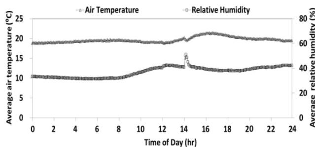
**Figure 3. Average indoor air temperature and RH on spraying days. Spraying was done at 14:00 h for 15 min at a dosage of 80 mL m<sup>-2</sup>.**
