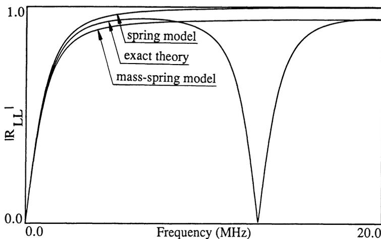
Fig. 3. Amplitudes of the normal incidence longitudinal-longitudinal reflection coefficient from a 0.1 mm thick epoxy layer between aluminium half-spaces. Comparison between the exact solution and the approximate theories.
