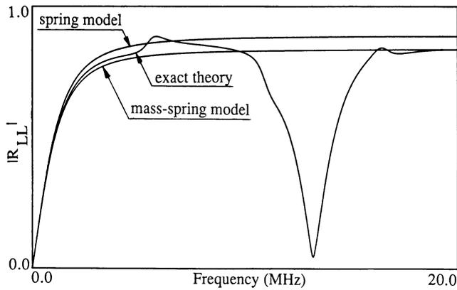
Fig. 4. Amplitudes of the longitudinal-longitudinal reflection coefficient from a 0.1 mm thick epoxy layer between aluminium half-spaces at an angle of incidence of 20 degrees. Comparison between the exact solution and the approximate theories.
