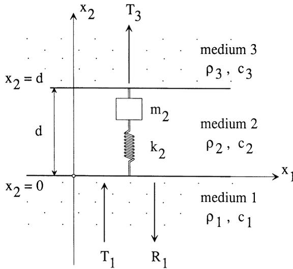
Fig. 2. Mass-spring approximation of a thin layer.
