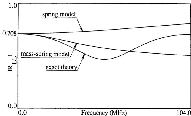
Fig. 5. Amplitudes of the normal incidence longitudinal-longitudinal reflection coefficients from a 50  $\mu\text{m}$  thick oxide layer between aluminium and epoxy half-spaces. Comparison between the exact solution and the approximate theories.
