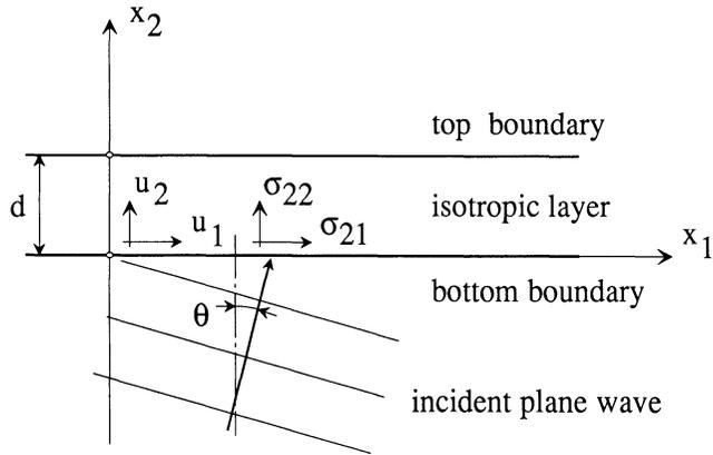
Fig. 1. Coordinate system position with respect to the layer. The infinite plane wave of frequency  $\omega$  strikes the layer at an angle of incidence  $\theta$ .
