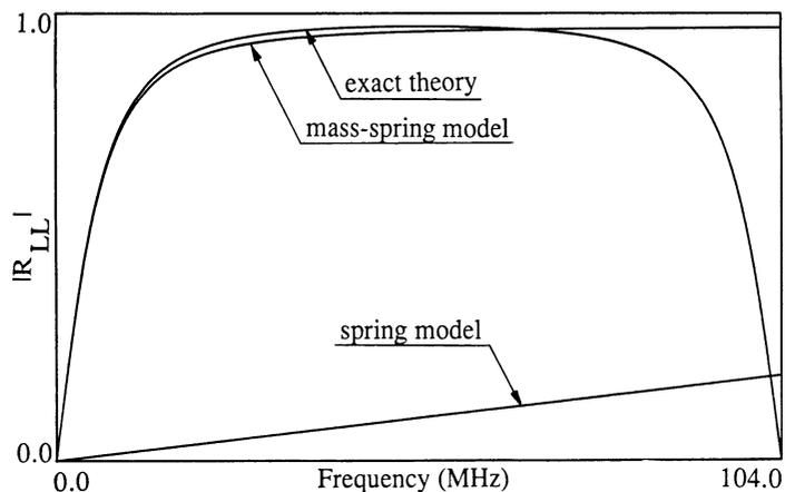
Fig. 6. Amplitudes of the normal incidence longitudinal-longitudinal reflection coefficient from a 50  $\mu\text{m}$  thick oxide layer in water. Comparison between the exact solution and the approximate theories.
