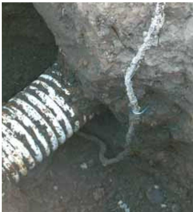
A macropore directly connects to a sub-surface drain. A polymer resin was poured from the surface, and then the soil was excavated around the macropore. (Photo courtesy of Martin Shipitalo, USDA-ARS, Coshocton, Ohio, USA)
