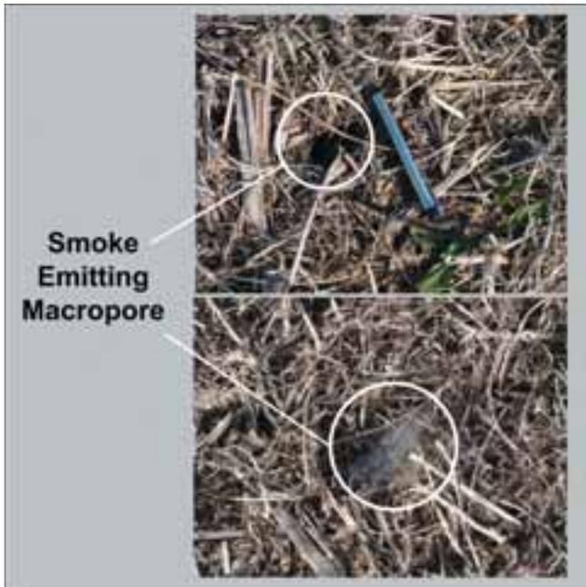
**Directly connected macropore emits smoke during a trial smoke-test experiment at the ISU Nashua Research Experimental Station. (Photo by Jorge Guzman, OSU)**
