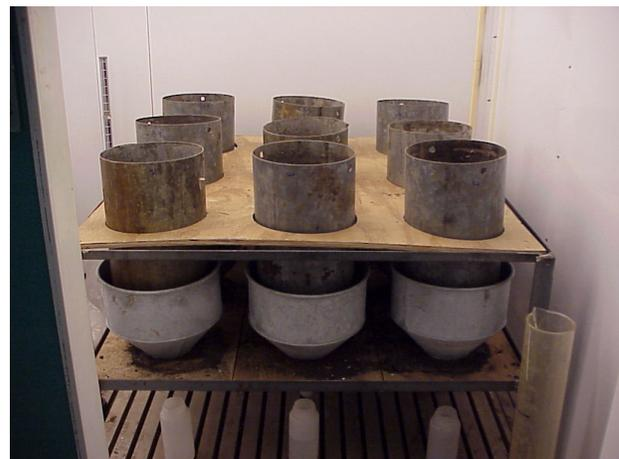
**Figure 1. Soil columns in the leachate collection apparatus.**
