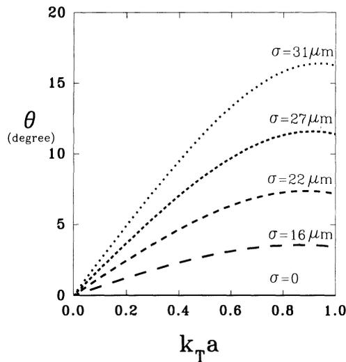
Fig. 3 Phase of the reflection coefficient vs. frequency for various roughness
