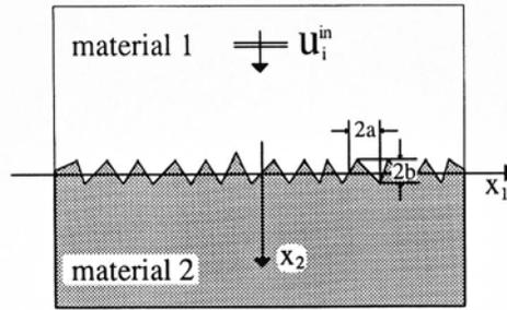
Fig. 1 A rough interface between dissimilar materials
