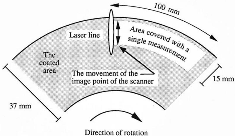
Fig. 1. The arrangement of measurement.
