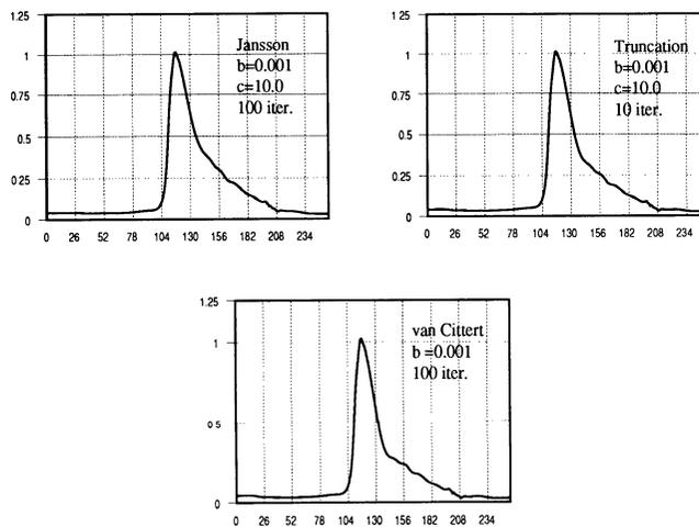
Fig. 3. Results of using Jansson's, truncation and van Cittert's iteration algorithms.
