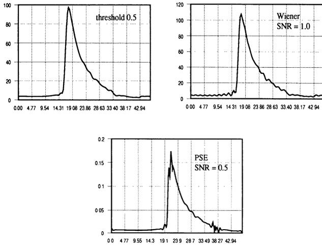
Fig. 2. Results of inverse, Wiener and PSE filtering.
