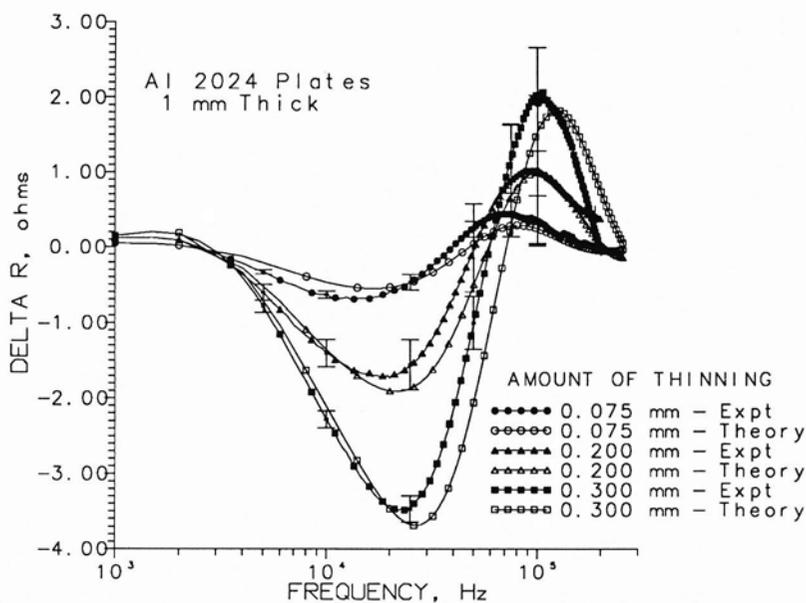
Fig. 3. Change in the real part of eddy-current probe impedance as a function of frequency for simulated corrosion at the bottom of the first layer of lap joint for 7.5, 20, and 30% metal loss. Open symbols are theoretical predictions; solid symbols represent mean of five independent measurements.
