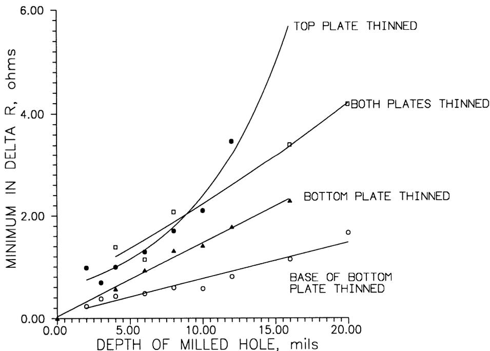
Fig. 4. Calibration curves showing strength of the minimum in the  $\Delta R$  vs. frequency curve plotted against depth of the milled region for each of the four sample orientations studied.
