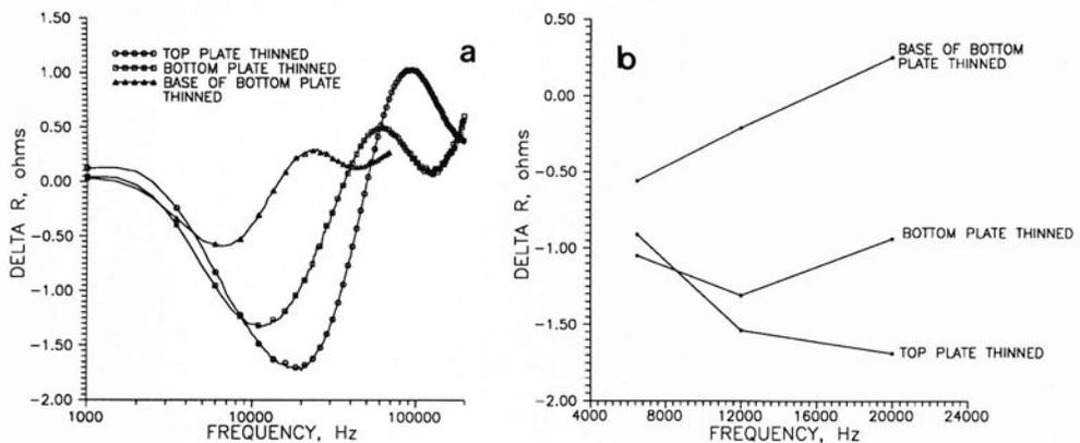
Fig. 5. Change in the real part of eddy-current probe impedance as a function of frequency for specimen milled to a depth of 0.2 mm with simulated metal loss located at different positions in lap joint. Complete impedance spectra (left) and value of  $\Delta R$  at three selected frequencies (right).
