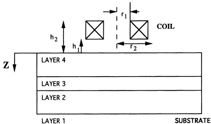
Fig. 1. Diagram of eddy-current coil geometry and structure of lap joint.
