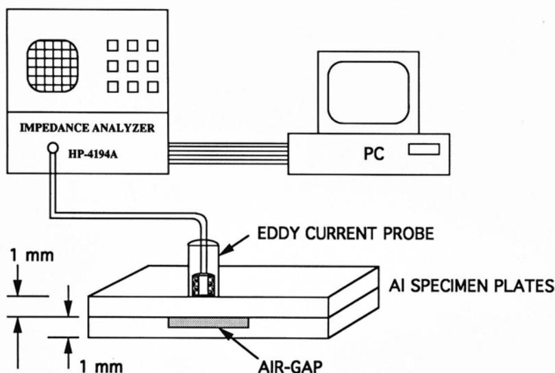
Fig. 2. Experimental apparatus used to measure impedance of eddy-current coil over simulated lap joint.
