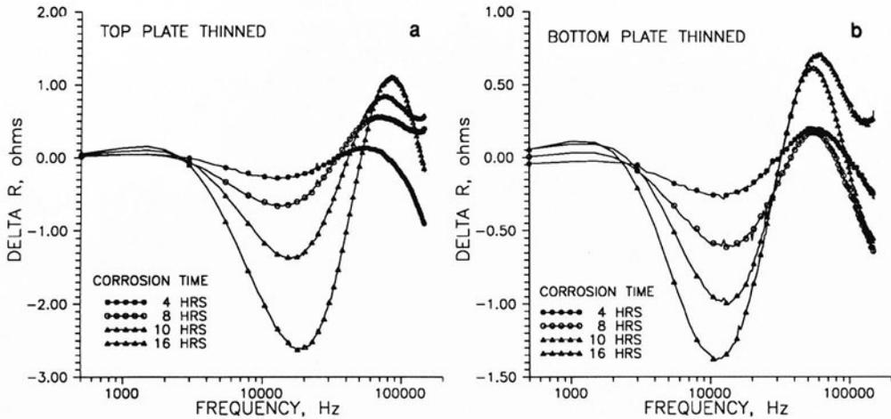
Fig. 6. Change in the real part of eddy-current probe impedance as a function of frequency for 2024 aluminum plates corroded electrochemically in NaCl solution for various times. Corroded region located at bottom of first layer (left) and at top of second layer (right).
