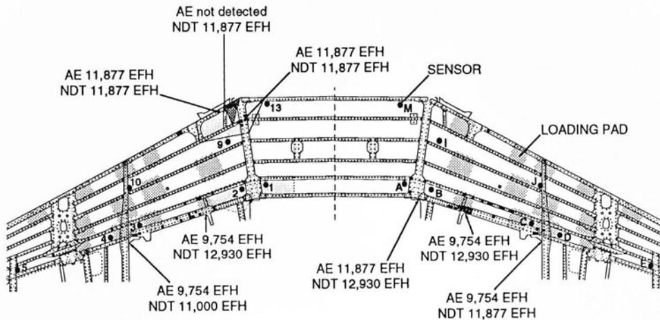
Fig. 2. Fatigue crack detection by continuous acoustic emission monitoring during 3,000 equivalent flying hours of full-scale testing. The numbers indicate the equivalent flying hours (EFH) at which acoustic emission detection or NDI confirmation took place. These defects occurred principally on the edge of the wing skin. Note that acoustic emission often detected the defect several thousands of equivalent flying hours before NDI confirmation was possible.
