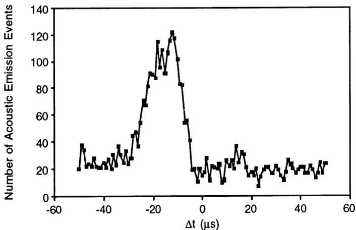
Fig. 5 Determination of crack site near sensor 3 (Fig. 2) by continuous acoustic emission monitoring. The measured acoustic velocity in the vicinity of this defect is  $0.5 \text{ cm}/\mu s$  and the halfwidth of the acoustic emission peak is  $16 \mu s$ . Linear zone location of the source is to within  $\pm 2 \text{ cm}$ .
