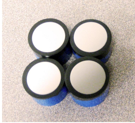
Figure 2.1 Samples that were cut, mounted, ground and polished.
