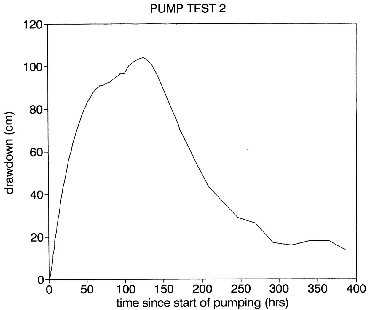
Figure 8. Pump test 2 MW-1 drawdown response and recovery
