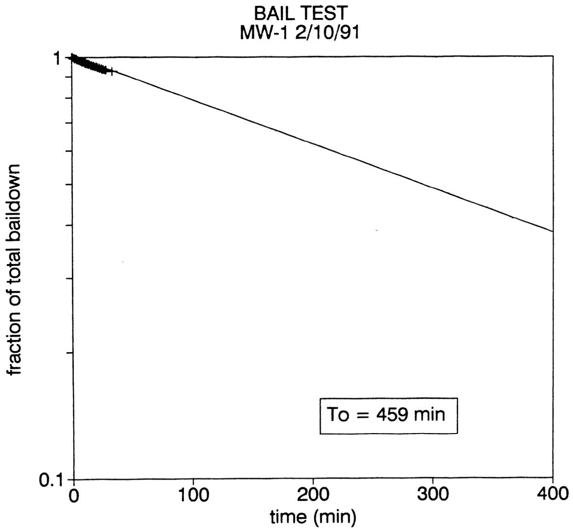
Figure 16. MW-1 bail test recovery vs. time and least squares fit
