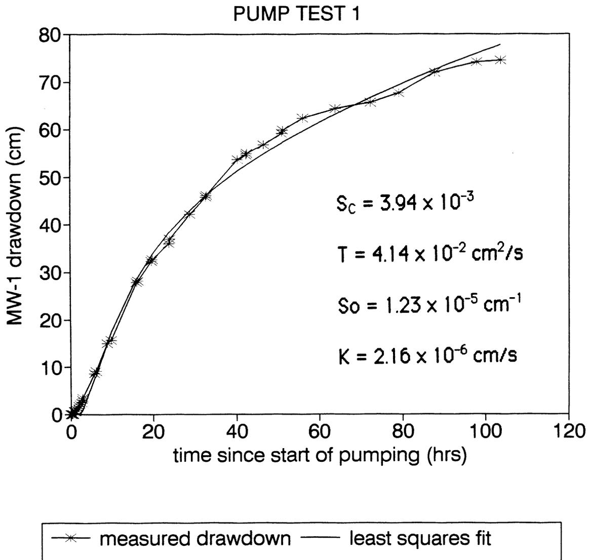
Figure 9. Pump test 1 drawdown in MW-1 vs. time and Theis solution least squares fit
