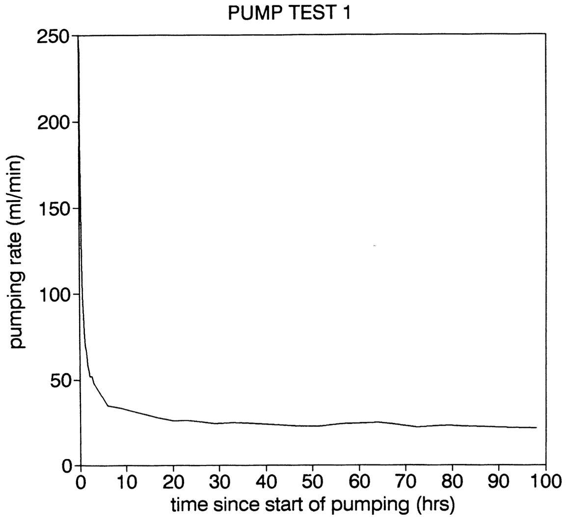
Figure 5. Pump test 1 pumping rate versus time
