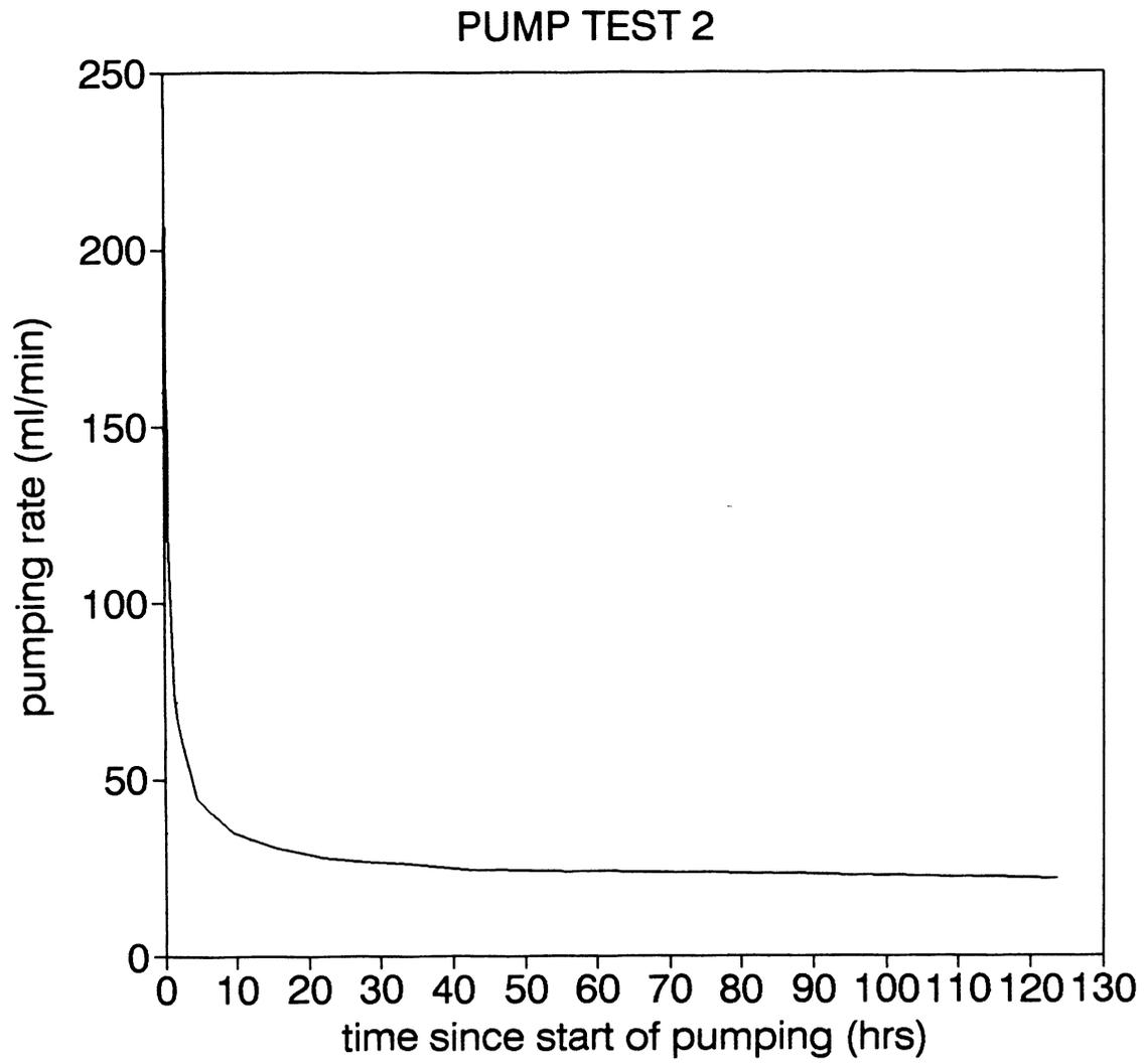
Figure 7. Pump test 2 pumping rate versus time
