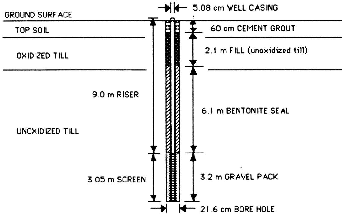
Figure 3. Vertical cross-section of wells IW-1 and MW-1 (not to scale)
