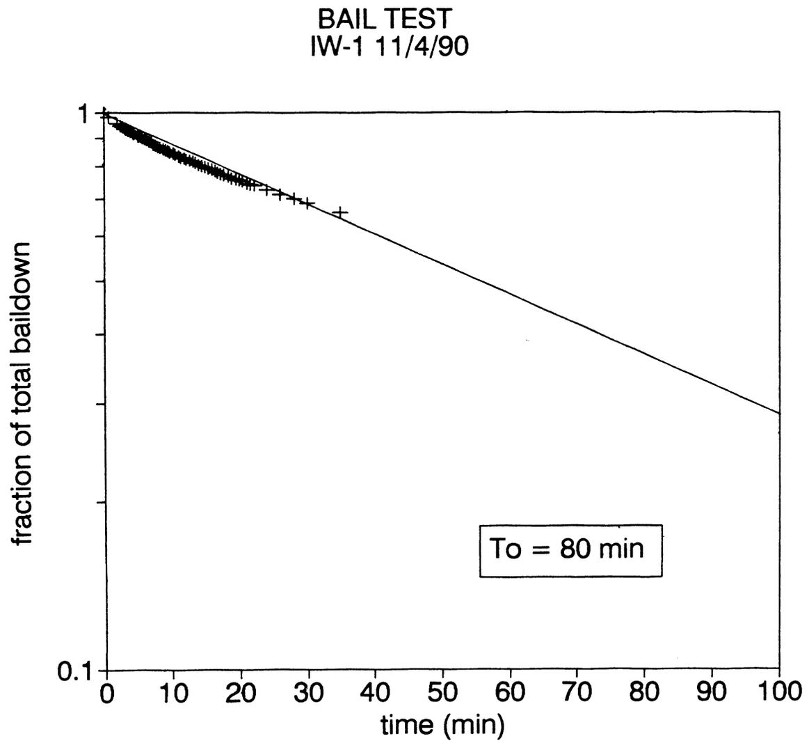
Figure 13. IW-1 bail test recovery vs. time and least squares fit
