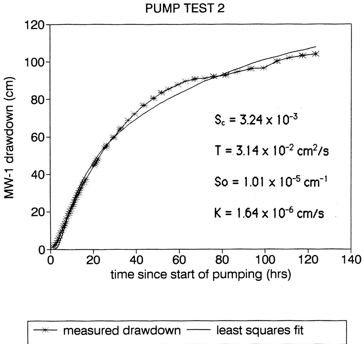
Figure 10. Pump test 2 drawdown in MW-1 vs. time and Theis solution least squares fit
