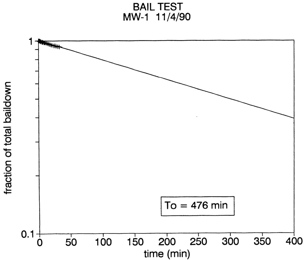
Figure 14. MW-1 bail test recovery vs. time and least squares fit
