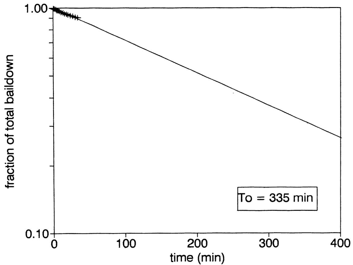
Figure 12. MW-1 predevelopment bail test recovery vs. time and least squares fit
