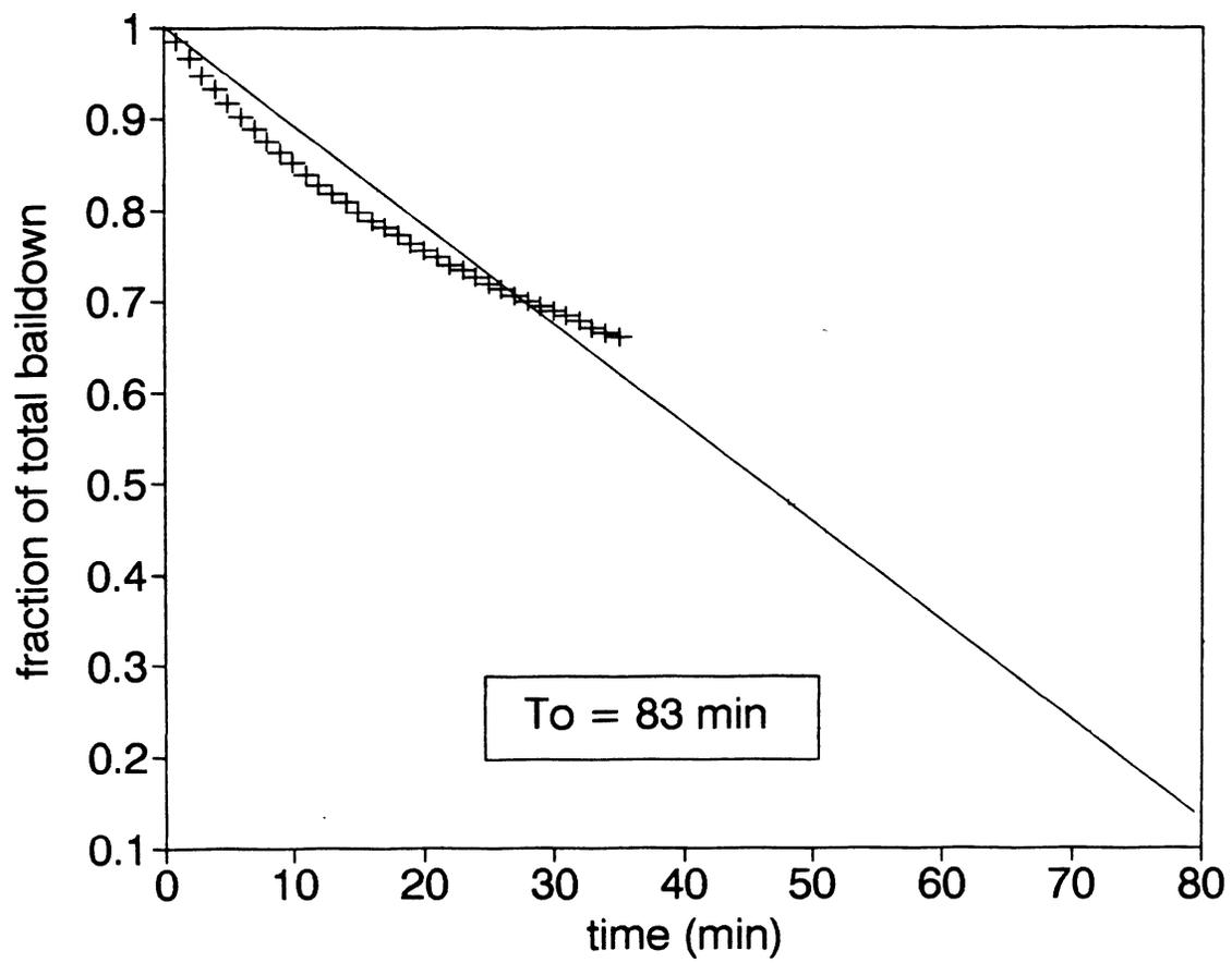
Figure 15. IW-1 bail test recovery vs. time and least squares fit
