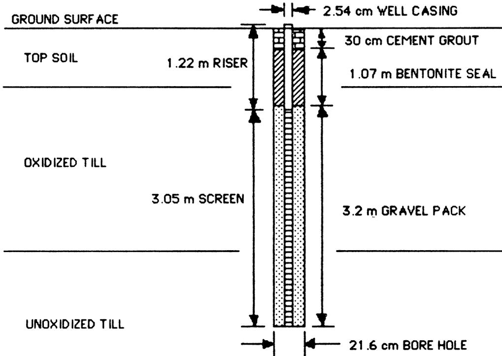
Figure 4. Vertical cross-section of well SW-1
