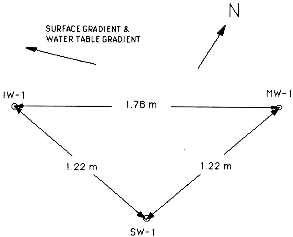
Figure 2. Plan view of the well layout. IW-1 & MW-1 are screened from 9.02 to 12.07 meters, SW-1 is screened from 1.16 to 4.21 meters. (scale: 1 inch = 0.39 meters)
