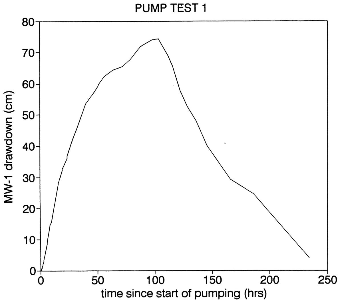
Figure 6. Pump test 1 MW-1 drawdown response and recovery
