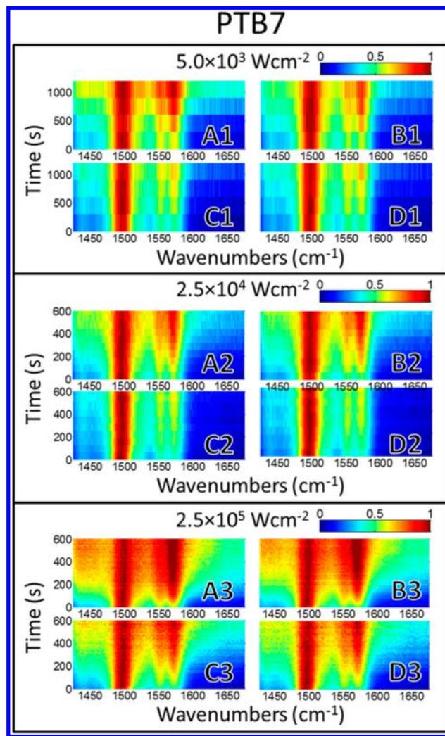
**Figure 6.** An expanded view of normalized PTB7 Raman spectra versus illumination time for three laser power densities listed above each set of graphs. Thick film with solvent evaporation under nitrogen (A1–A3), thick film with slow solvent evaporation under nitrogen (B1–B3), thin film with solvent evaporation under nitrogen (C1–C3), and a thin film dried under nitrogen followed by thermal annealing (D1–D3). The color scale is Raman scattering intensity.
