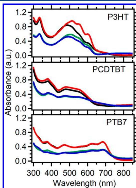
Figure 2. Absorption spectra for P3HT, PCDTBT, or PTB7 samples with the following preparation: thick film with solvent evaporation under nitrogen (black); thick film with slow solvent evaporation under nitrogen (red); thin film with solvent evaporation under nitrogen (blue); and a thin film dried under nitrogen followed by thermal annealing (green). Other sample preparation and thicknesses are shown in Table 1
