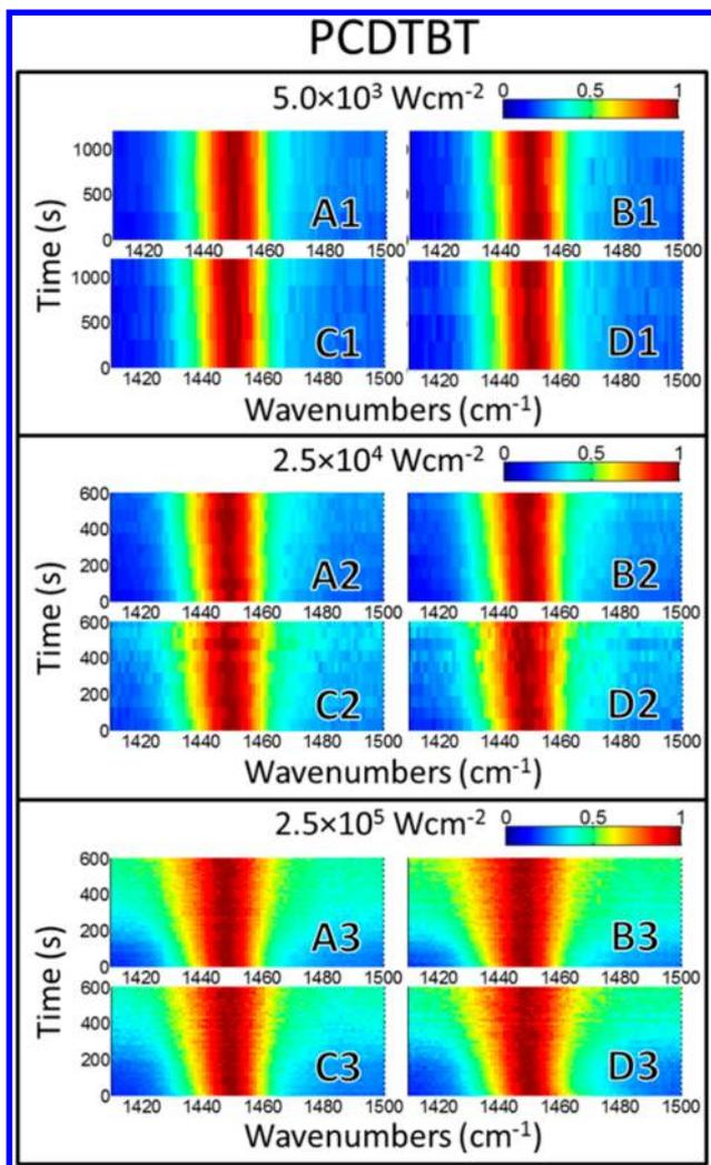
**Figure 5.** An expanded view of normalized PCDTBT Raman spectra versus illumination time for three laser power densities listed above each set of graphs. Thick film with solvent evaporation under nitrogen (A1–A3), thick film with slow solvent evaporation under nitrogen (B1–B3), thin film with solvent evaporation under nitrogen (C1–C3), and a thin film dried under nitrogen followed by thermal annealing (D1–D3). The color scale is Raman scattering intensity.
