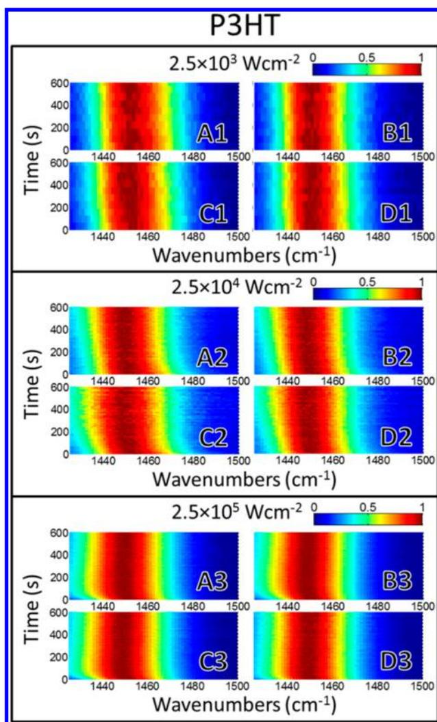
**Figure 4.** An expanded view of normalized P3HT Raman spectra versus illumination time for three laser power densities listed above each set of graphs. Thick film with solvent evaporation under nitrogen (A1–A3), thick film with slow solvent evaporation under nitrogen (B1–B3), thin film with solvent evaporation under nitrogen (C1–C3), and a thin film dried under nitrogen followed by thermal annealing (D1–D3). The color scale is Raman scattering intensity.
