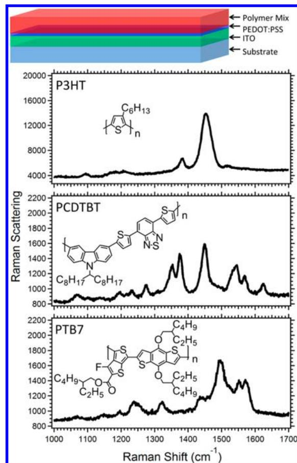
**Figure 1.** At the top is a schematic of the sample layout. Raman spectra of samples formed with the donor P3HT, PCDTBT, or PTB7 (as indicated by the label and structure) mixed with PC<sub>x</sub>BM. P3HT ( $180.6 \pm 0.7$  nm thickness), PCDTBT ( $180 \pm 10$  nm), and PTB7 ( $160 \pm 10$  nm) films were prepared with solvent evaporation under nitrogen and measured with  $2.5 \times 10^3$  (P3HT) or  $5.0 \times 10^3$   $\text{Wcm}^{-2}$  (PCDTBT and PTB7).
