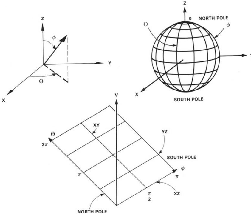
Fig. 4 — Schematic diagram showing mapping of velocity surfaces.
