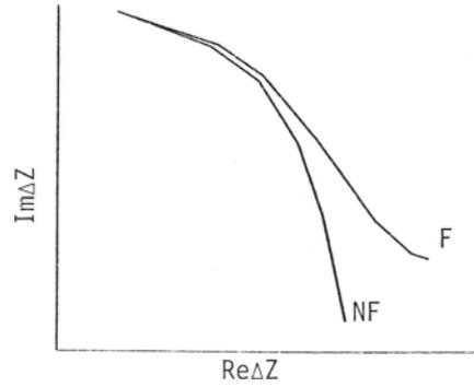
Fig. 4. Impedance loci for the scan shown in Fig. 3. The impedance change  $\Delta Z$  is the change relative to the probe impedance in free space;  $F$  and  $NF$  refer to scans with and without the flaw indicated in Fig. 3.
