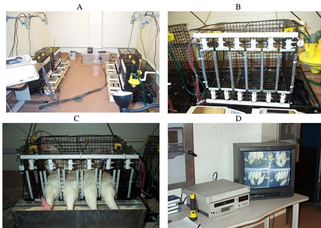
**Figure 1. Photo views of the experimental setup: testing room (A); close-up view of feeder access openings with IR sensor pairs above and below each opening (B); hens feeding through instrumented feeder openings (C); video display and recording system (D).**
