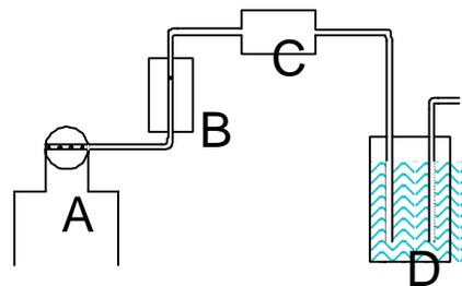
Figure 4. Schematic of NH<sub>3</sub> sampling flow path during application (not to scale): A – hood enclosing injector; B – rotometer; C – air pump; D – collection bottle with acid solution. Intake tube in area above A is shown in figure 3.
