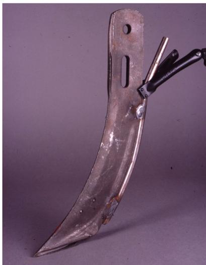
**Figure 2.** Knife used to inject NH<sub>3</sub>.
