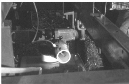
Figure 3. Top of hood over injector showing air exit from suction fan. Small tube inside air exit draws sample air used to measure NH<sub>3</sub> loss.
