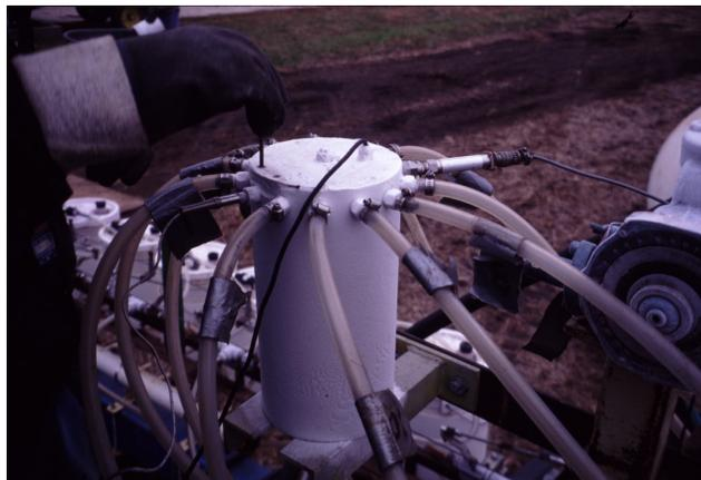
Figure 1. Old Impellicone manifold.
