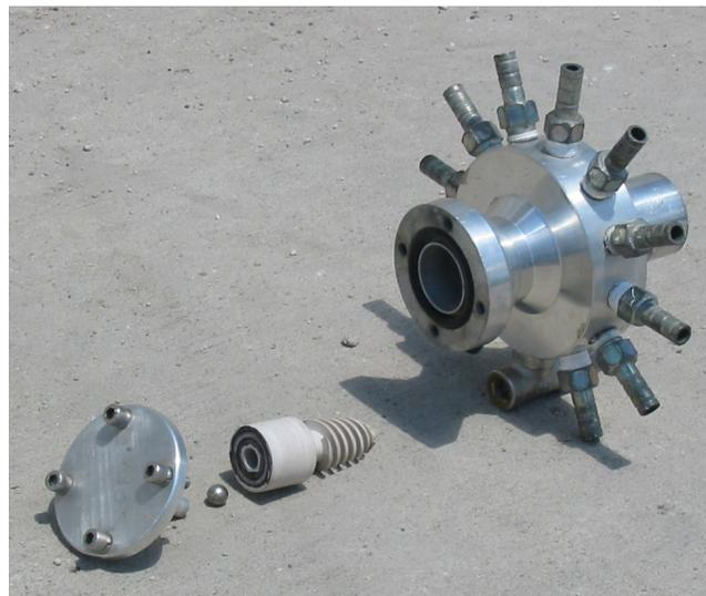
Figure 4. Exploded view of new Impellicone manifold showing lid, ball bearing, cone, and body (left to right).
