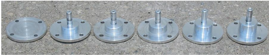
Figure 5. Lid styles (left to right): smooth lid, 16.38-mm (0.645-in.), 18.54-mm (0.730-in.), 20.68-mm (0.814-in.), 24.13-mm (.950-in.) (not used in this experiment), and 27.56-mm (1.085-in.) lids.
