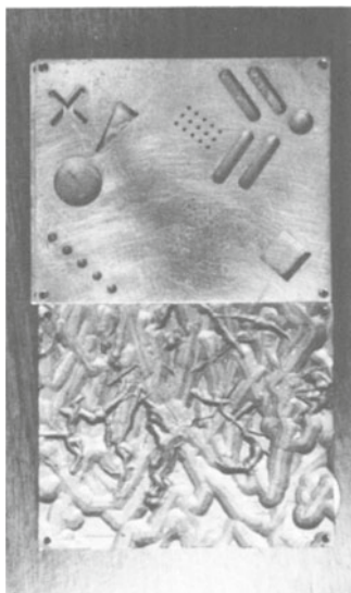
Fig. 8. Top: Copper portion of copper/steel phantom. Bottom: Steel plate of copper/steel phantom.
