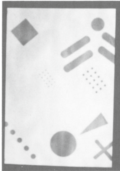
Fig. 9. Radiogram of copper/steel phantom at 0 degrees, taken in 25 minutes.
