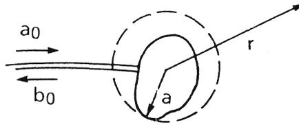
Fig. 2. General immersion transducer with feeding cable.
