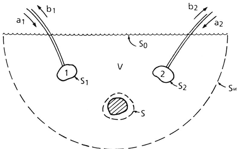
Fig. 1. Generic pitch-catch, immersion measurement.
