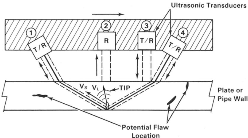
Fig. 1. Four transducer array configuration.
