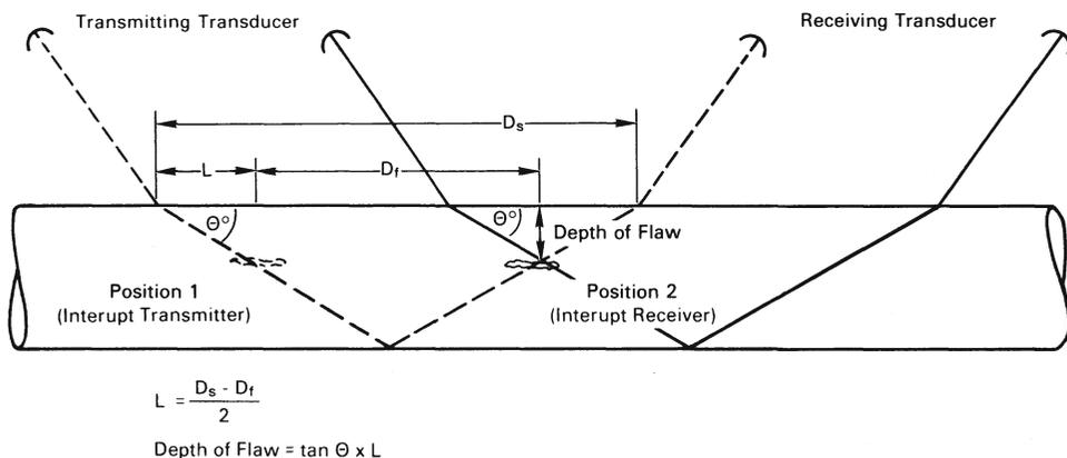
Fig. 2. Triangulation for location (depth) calculation.
