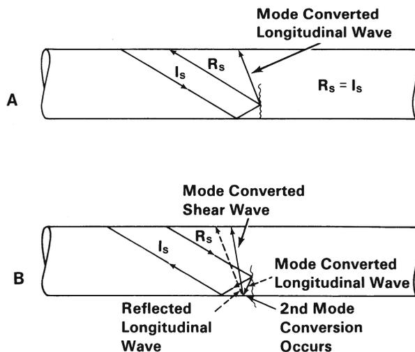
Fig. 3. A and B: Mode converted signal sources.
