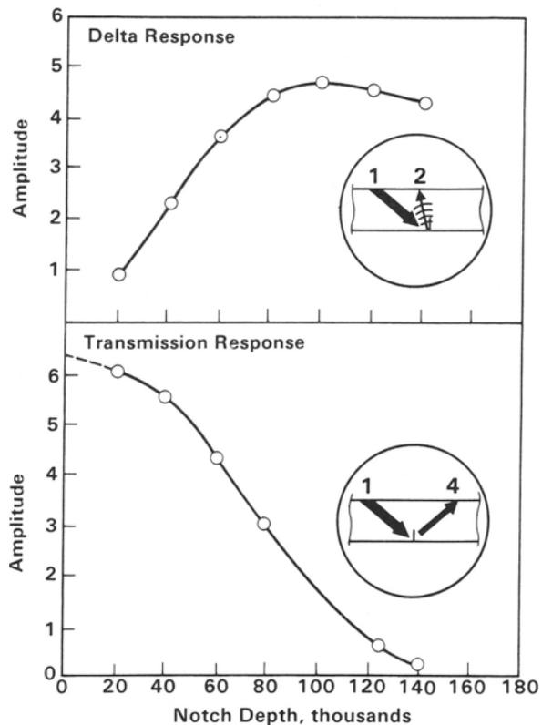
Fig. 4 Response from the four transducer array.
