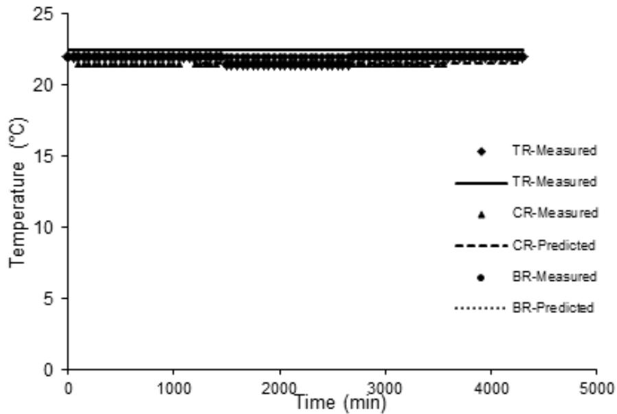
**Figure 6.** Measured and predicted maize room temperature changes over time at room temperature in the vertical direction (before the freezing experiments). TR= Top room, CR= center room, BR = bottom room.
