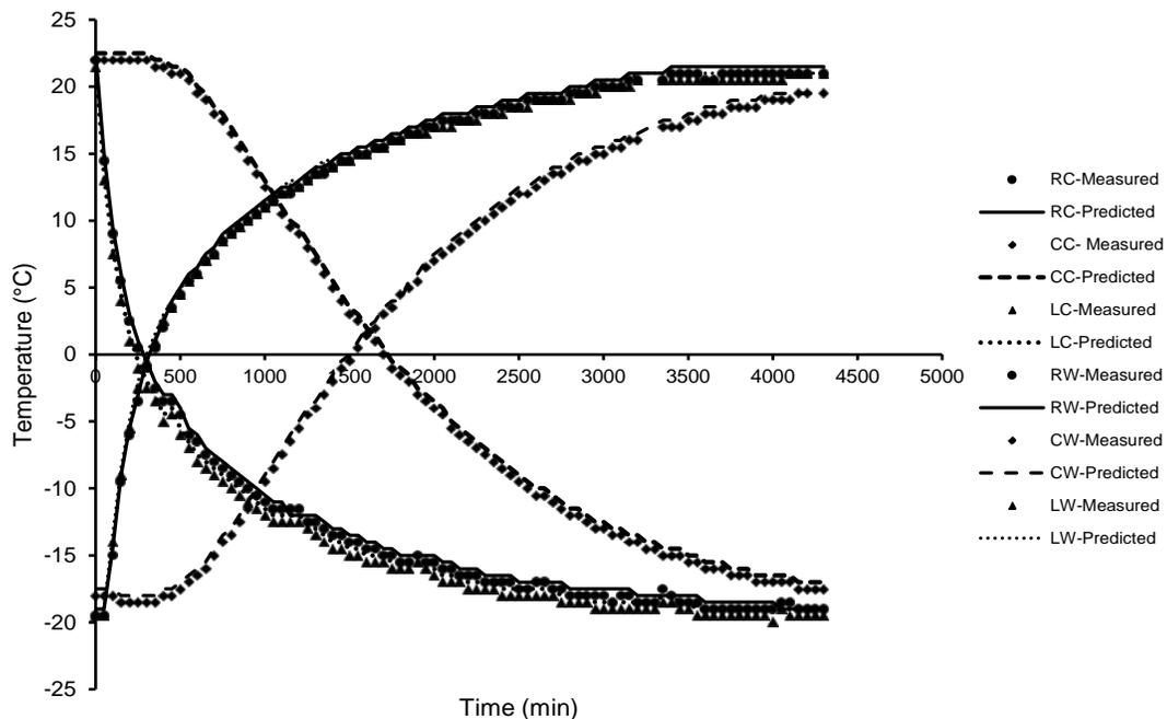
**Figure 9.** Measured and predicted maize grain temperature change over time from room to freezing temperature and from freezing to room in the radial direction. TW= Top warming, CW= center warming, BW = bottom warming, TC = top cooling, CC = center cooling and BC= bottom cooling.
