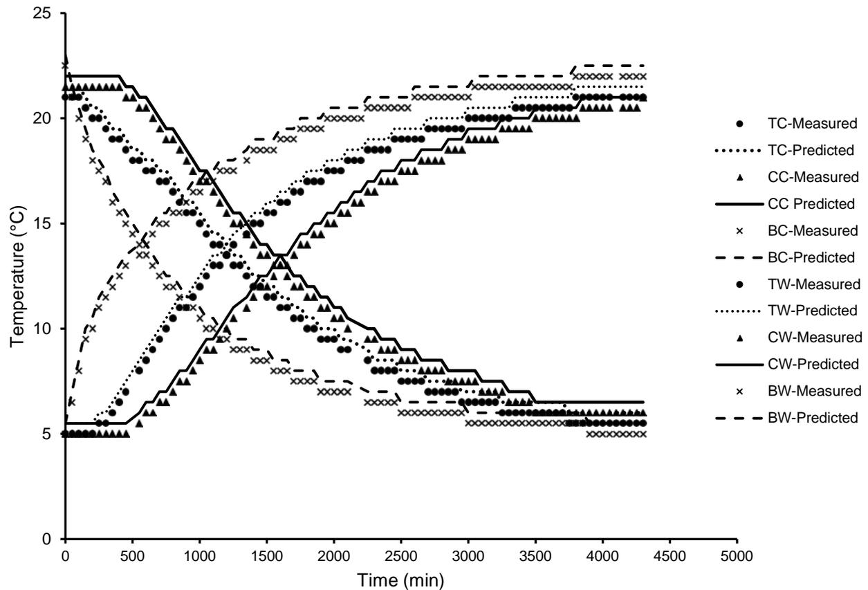
**Figure 3.** Measured and predicted maize grain temperature over time from the room to cooler and from cooler to back room temperature in the vertical direction. TC = Top cooling, CC= center cooling, BC= bottom cooling, TW = top warming, CW= CENTER warming, BW= bottom warming.
