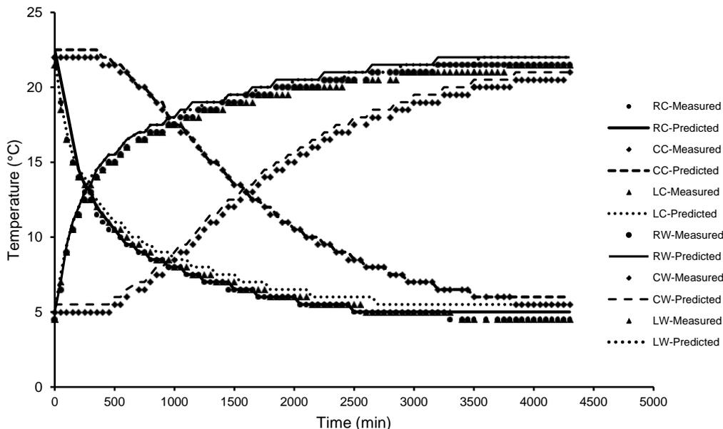
**Figure 5.** Measured and predicted maize grain temperature over time from the room to cooler and from cooler to back room temperature in the radial direction. RC= Right cooling, CC= center cooling, LC= left cooling, RW= Right warming, CW= center warming, LW=left warming.
