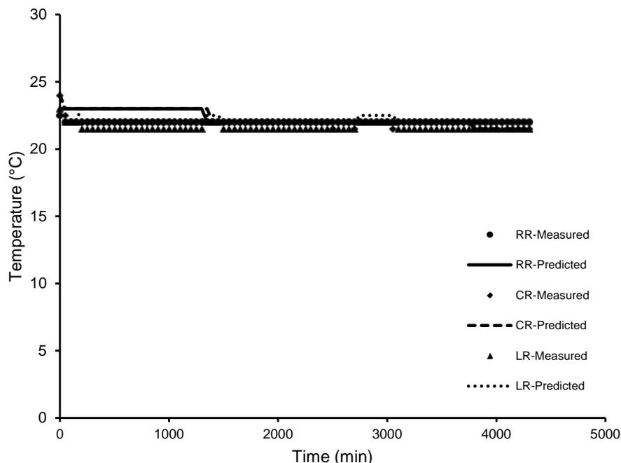
**Figure 8.** Measured and predicted maize grain room temperature change over time at room temperature in the radial direction (before the freezing experiments). RR= Right room, CR= center room, LR= left room.
