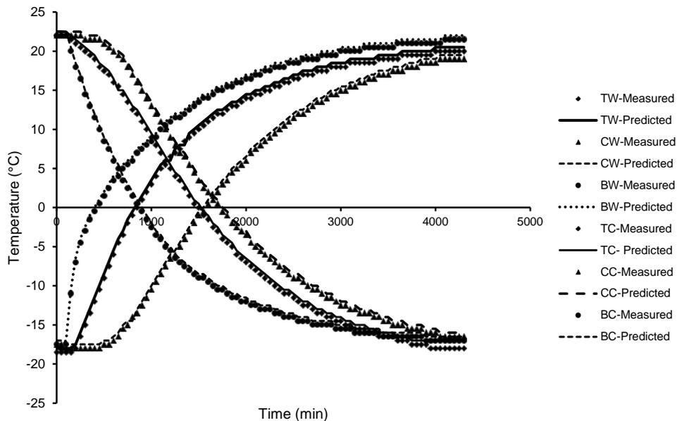
**Figure 7.** Measured and predicted maize grain temperature change over time from room to freezing temperature and from freezing to room in the vertical direction. TW= Top warming, CW= center warming, BW= bottom warming, TC= top cooling, CC= center cooling and BC= bottom cooling.
