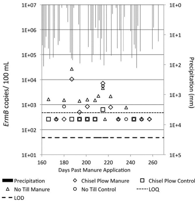
**Fig. 1.** *ErmB* concentrations in tile drainage water following manure application in plots under no-till and chisel plow regimes with LOQ and LOD. Concentrations less than the LOQ and greater than LOD were assigned the average value of the LOQ and LOD for visualization.
