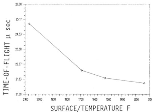
Fig. 8. Time-of-flight versus temperature for the 316 stainless steel continuous cast billet 22 feet from the mold. Data taken at the end of the cast when the billet is stationary for several minutes.
