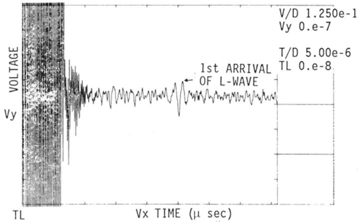
Fig. 6. Pulsed EMAT receiver response for a 4x4 in. 316 continuous cast steel billet 22 feet from the mold. Surface temperature 2070°F.
