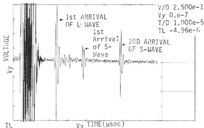
Fig. 5. Pulsed EMAT receiver response for the 4 inch, fine-grained 304 stainless steel calibration block
