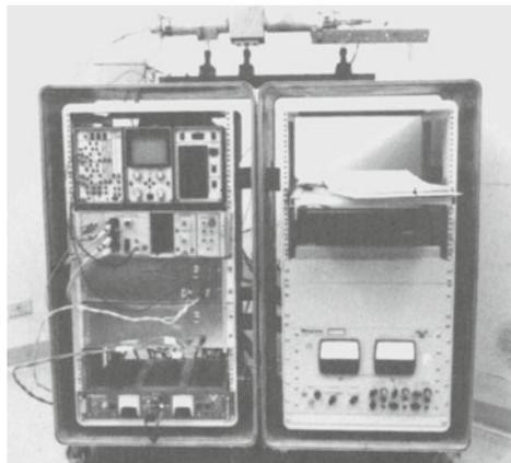
Fig. 2. High temperature pulsed EMAT system packaged for in-plant demonstration
