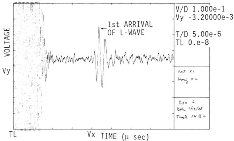
Fig. 7. Pulsed EMAT receiver response for a 4x4 in. 304 continuous cast steel billet after the flame torch cut-off. Surface temperature 1200°F.
