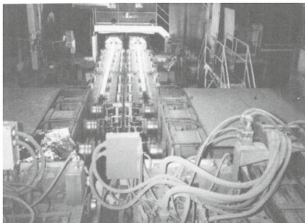
Fig. 1. Beginning of continuous cast run showing the mold face of the continuous caster at the Baltimore Specialty Steel Corporation plant
