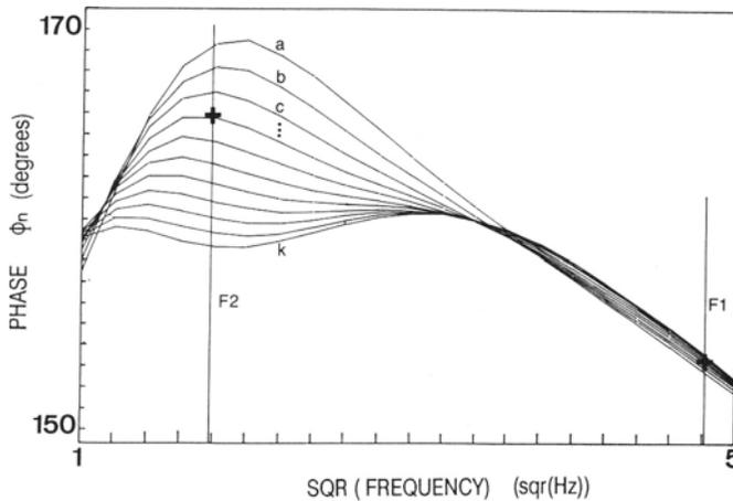
Fig. 3. Titanium pipes characterization: Phase of the normal Mirage deflection versus the square root of the frequency. The different curves are deduced from calculation of the phase for different thicknesses of the air slice:
