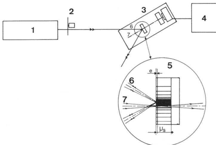
Fig. 1. Experimental set up of optical losses determination in coatings using the colinear mirage detection.
