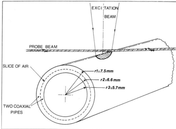
Fig. 2. Titanium pipes sample study with the disposition of the two beams of the Mirage detection.
