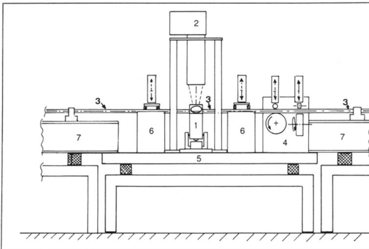
Fig. 4. Central part of the machine for the test of titanium pipes :
