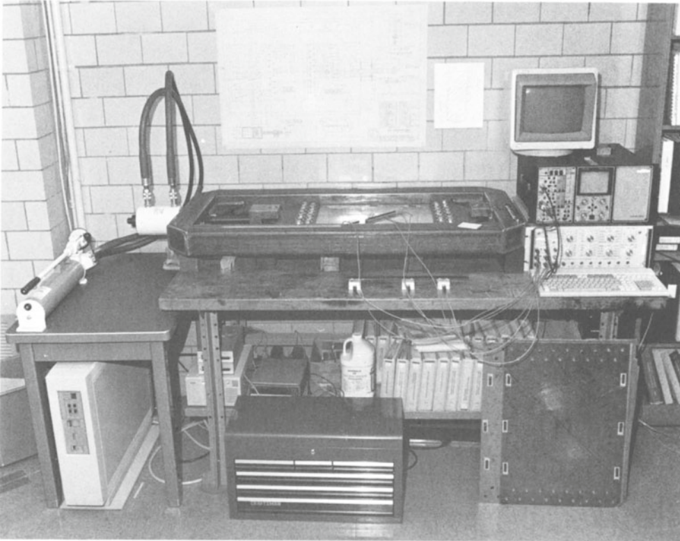
Fig. 1. Load frame and equipment for the ultrasonic measurement of stress in the presence of texture on metal plate.
