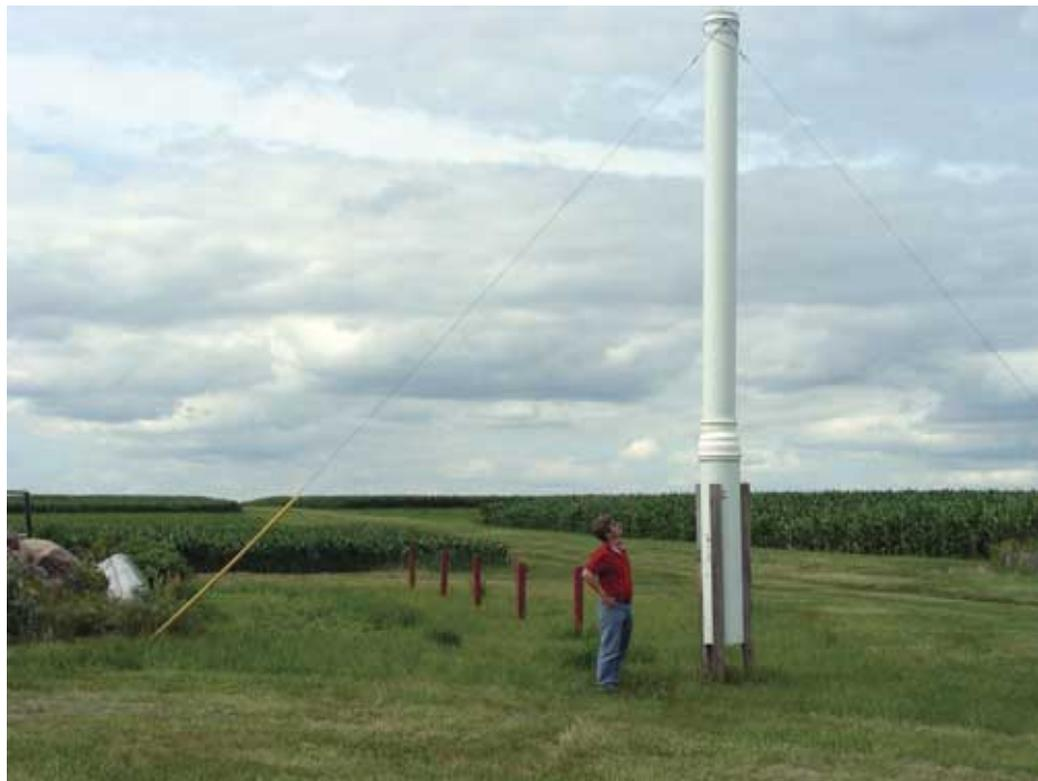
*One of four suction traps set up in Iowa in 2005 for soybean aphid sampling. The traps are approximately 20 feet tall to collect winged aphids that are migrating from buckthorn to soybean and back. At this size, the traps are unlikely to collect aphids*
