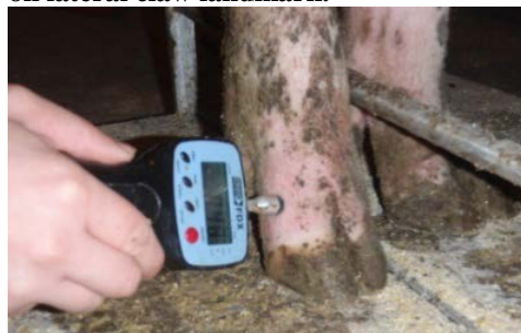
Figure 1. Mechanical Nociception Threshold (MNT) test on lateral claw landmark.
