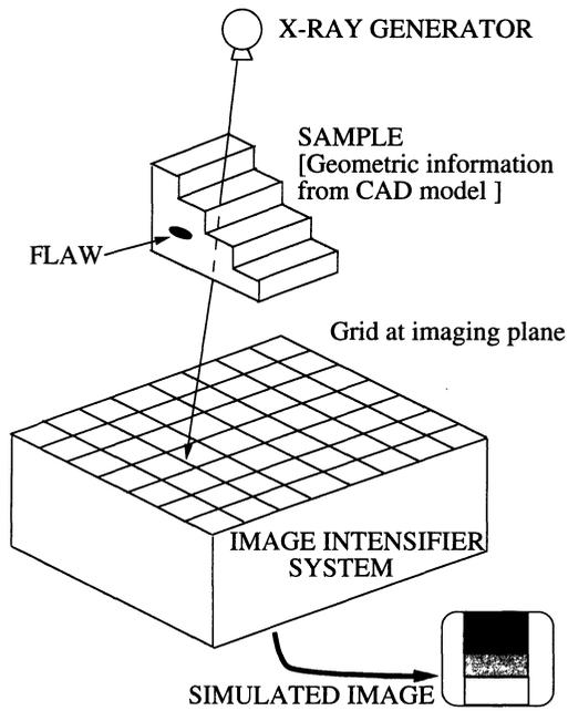
Fig. 1. Schematic overview of the RTSIM computer model.
