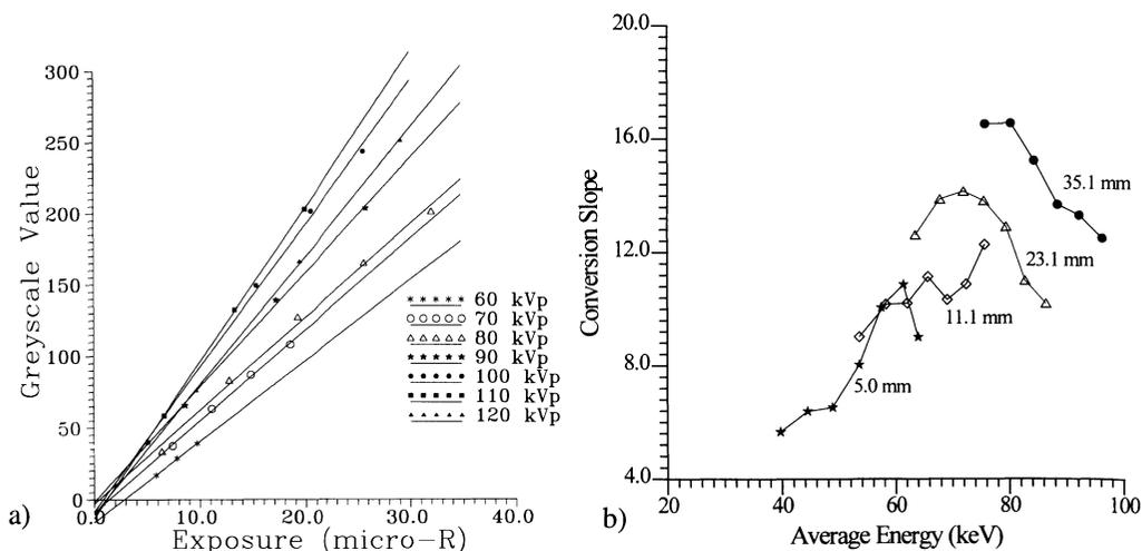
Fig. 3. a) Observed relation between greyscale value and exposure for transmission through 5.0 mm aluminum at different voltage settings. b) Correlation between the slope of the greyscale calibration curves and the average incident energy.
