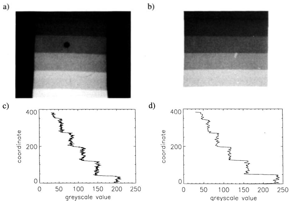
Fig. 4. a) Real, and b) simulated single-frame images of an aluminum step wedge varying in thickness from 5 mm to 20 mm in 3 mm steps. Profiles through the real, and simulated, image are shown in c), and d), respectively.
