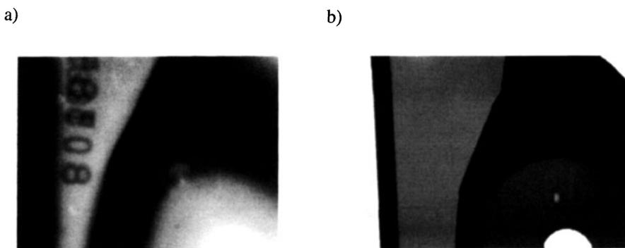
Fig. 6. a) Real, and b) simulated images of an iron casting. The simulated image contains a simulated ellipsoidal flaw located in the thin region above the hole.
