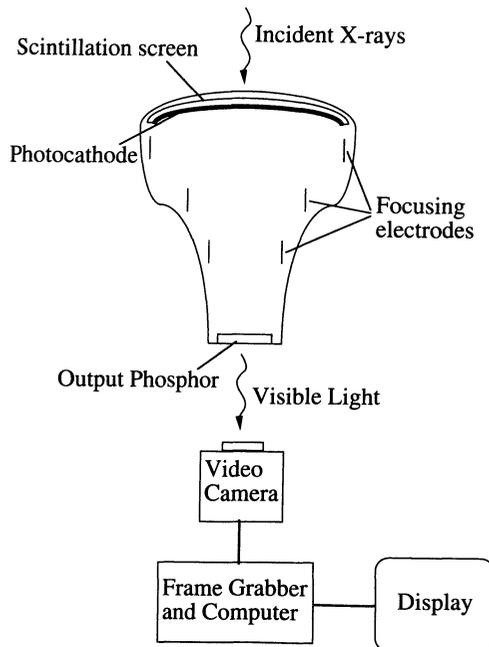
Fig. 2. Schematic representation of a typical real-time imaging system.
