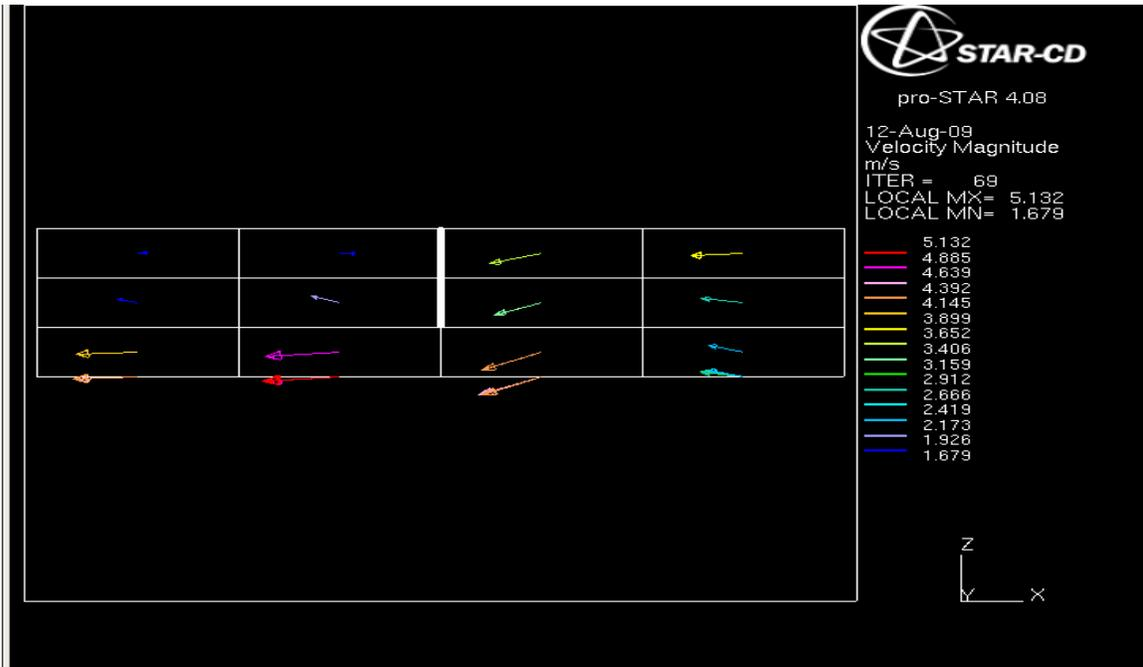
Figure 82 - Velocity magnitude around baffle at 3 cell depth
