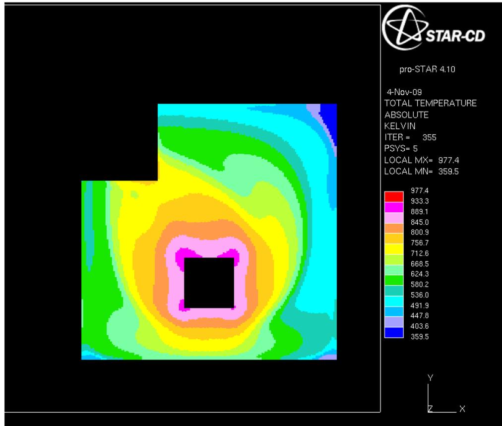
Figure 3 - High-fidelity model temperature profile with no baffles
