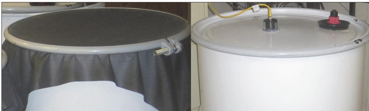
Figure 1. Barrels used for (left) non-hermetic and (right) hermetic storage.
