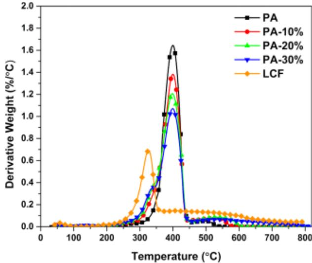
Figure 10. Weight derivative of pure PA polymer, LCF, and PA-LCF composites.
