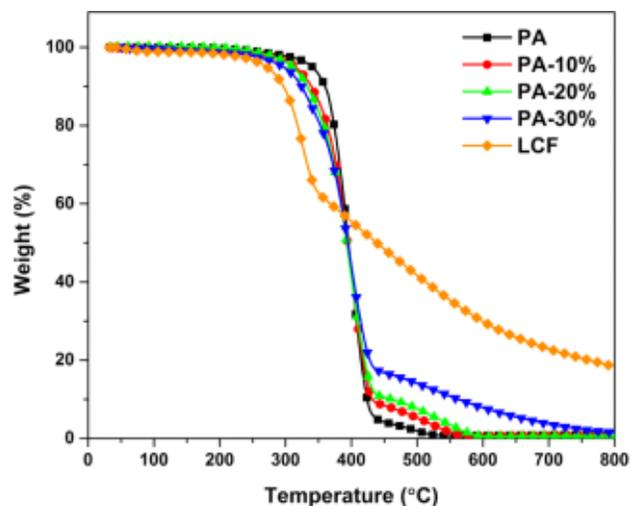
Figure 8. Thermal degradation behavior of pure PA polymer, pure LCF, and PA-LCF composites.
