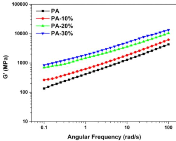
Figure 3. Angular frequency dependence of storage modulus at 140°C for PA-LCF composites containing different percentages of filler.
