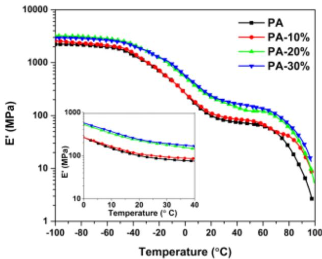
Figure 5. Storage modulus as a function of temperature for the pure PA polymers and its composites with 10 wt % to 30 wt % LCF.
