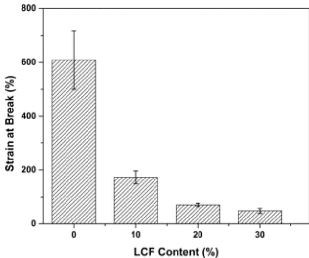
Figure 13. Strain at break as a function of LCF content.
