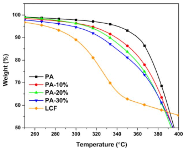
Figure 9. Enlarged portion of Figure 8 showing detail for the onset of thermal degradation.
