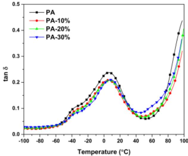
Figure 6.  $\tan \delta$  curves as a function of temperature obtained via DMA.
