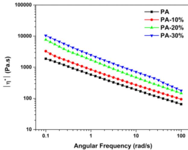
Figure 4. Angular frequency dependence of complex viscosity at 140°C for PA-LCF composites containing different percentages of filler.
