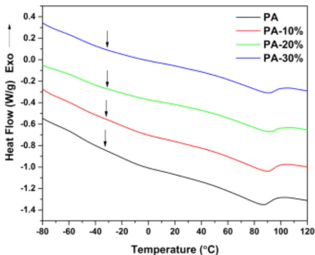
Figure 7. DSC traces of PA polymer and composites containing 10, 20, and 30 wt % of LCF.
