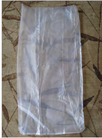
Figure 4: PICS 80- \mu m polyethylene inner bag řekil 4: PICS 80 mikron polietilen i uval
