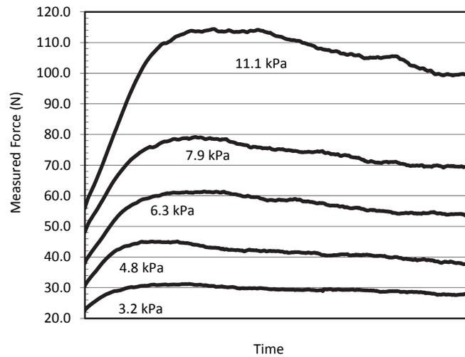
Figure 2. Typical example of measured force traces over time for the five normal grain pressures.
