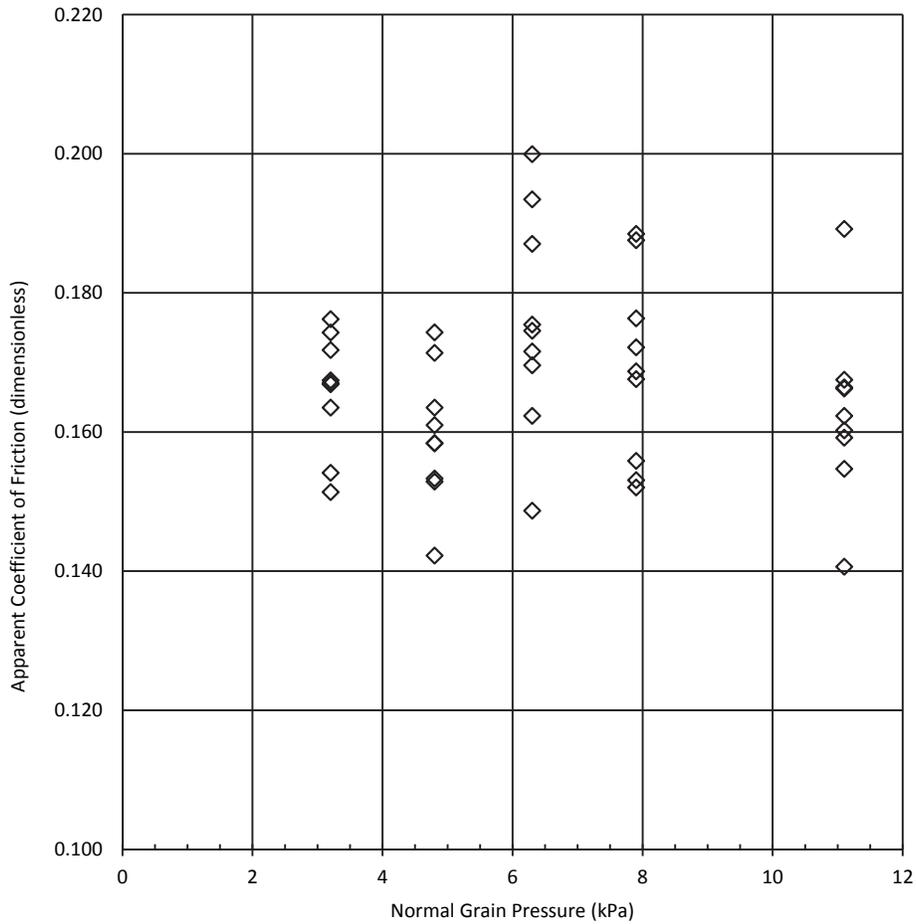
**Figure 3. Apparent coefficient of friction of wheat on denim for normal grain pressures.**
