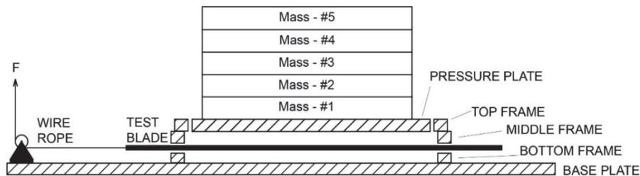
Figure 1. Schematic of the friction device used to measure the apparent coefficient of friction.
