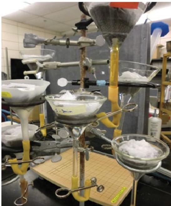
**Figure 1:** a) Ozone generator, reactor, and sample ozonation; b) Soaking of samples after ozonation in Baermann funnels for 24 h and 48 h and draw-off of the filtrate to collect viable nematodes for counting and assessment of treatment.
