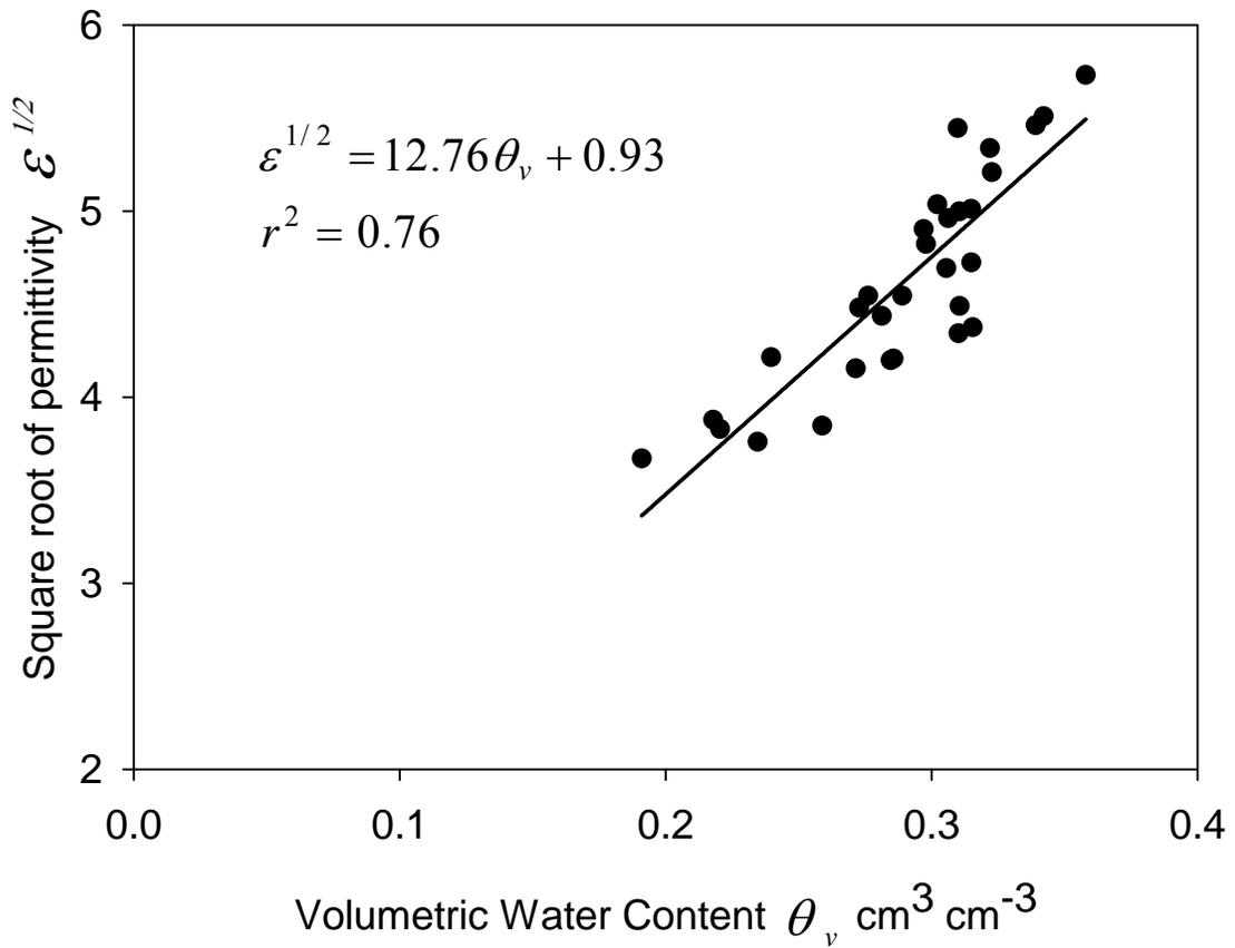
Figure 2.4. Field relationship between the square root of permittivity ( $\epsilon^{1/2}$ ) as measured by the PR2 probe and observed volumetric water content ( $\theta_v$ ) computed by gravimetric water content and bulk density.
