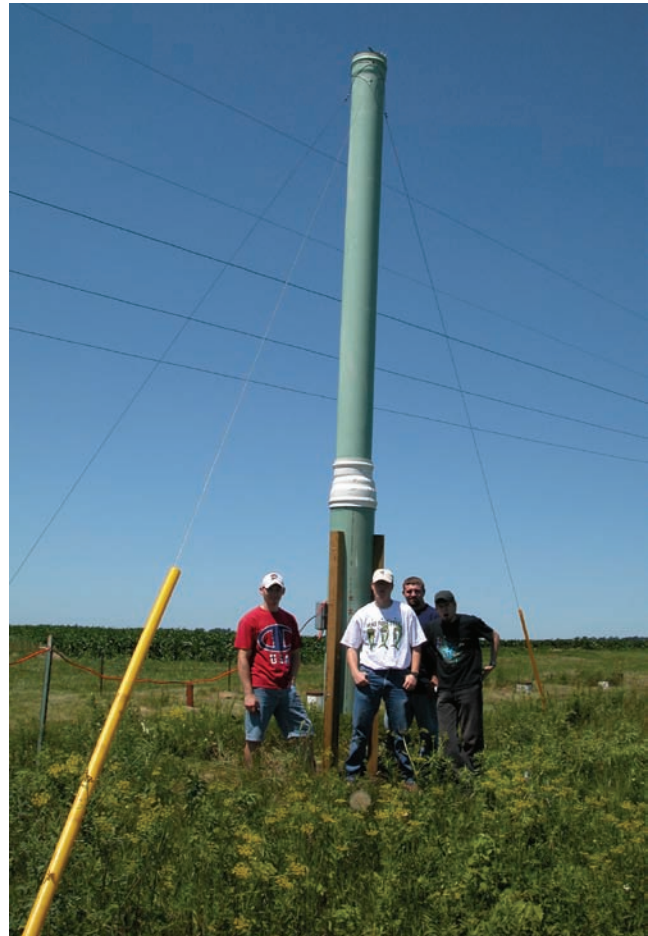
One of four suction traps set up in Iowa in 2005 for soybean aphid sampling. The traps are approximately 25 feet tall to collect winged aphids that are migrating from buckthorn to soybean and back. At this size, the traps are unlikely to collect aphids that fly from one soybean plant to another. Traps will be run from May through October during the 2006 growing season.
