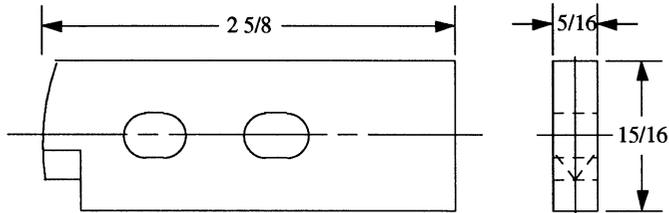
Fig. 1 The shape and dimensions of the workpiece (dimensions are inches).
