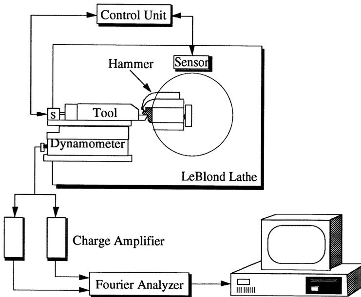
Fig. 2 Schematic diagram for machining experiments.
