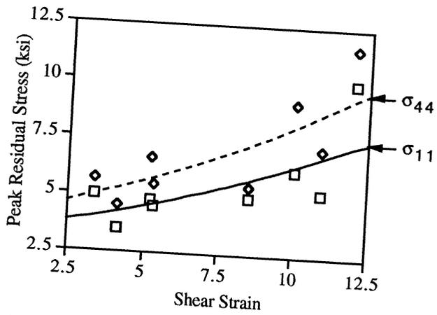
Fig. 5 Sensitivity of peak residual stress to shear strain.
