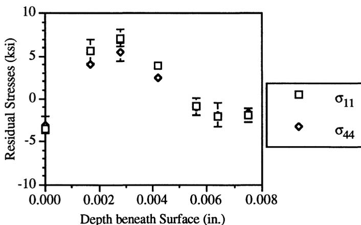
Fig. 3 Typical result of the residual stress distribution with the depth beneath the machined surface.
