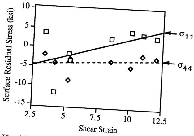
Fig. 4 Sensitivity of surface residual stress to shear strain.
