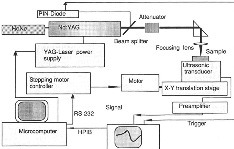
Fig. 1. Photoacoustic measurement setup.
