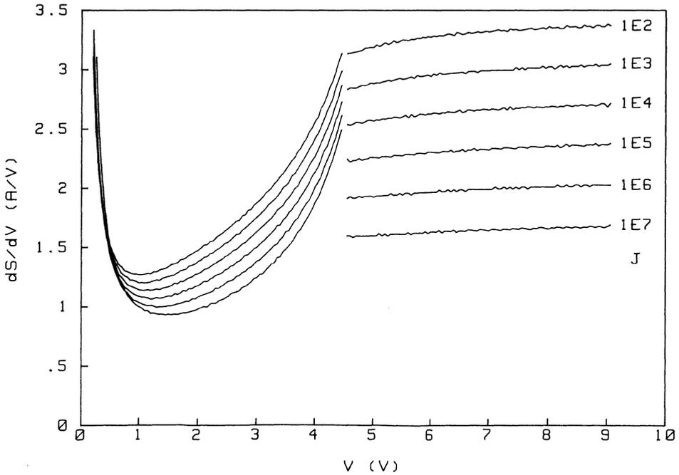
Fig. 4. Theoretical  $ds/dV$  versus  $V$  for constant  $J$  in  $\text{A}/\text{cm}^2$  from one-dimensional model of MIM junction,  $\phi_0=4.5$  eV.
