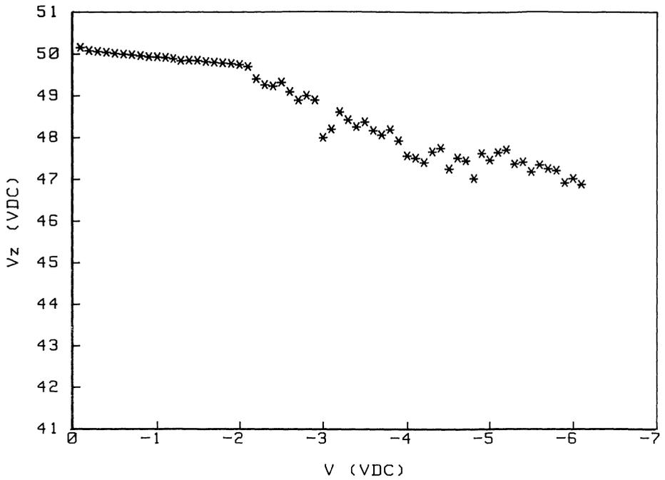
Fig. 1. Transducer voltage ( $V_z$ ) versus tip-sample voltage ( $V$ ) for a constant current ( $I$ ) of 2.7 nA: W tip, Pt sample.
