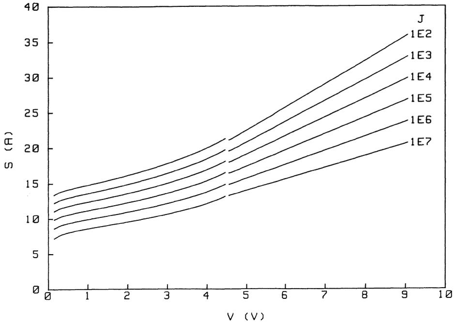
Fig. 3. Theoretical insulator thickness ( $s$ ) versus potential difference ( $V$ ) between metals for constant current density ( $J$ ) in  $\text{A}/\text{cm}^2$  from one-dimensional model of MIM junction,  $\phi_0=4.5$  eV.
