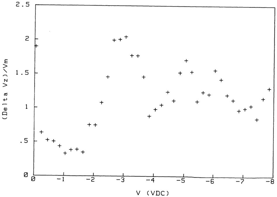
Fig. 2. Change in transducer voltage ( $\Delta V_z$ ) divided by tip-sample modulation voltage ( $V_m$ ) versus  $V$  for a constant current ( $I$ ) of 10.7 nA,  $f=50.1$  Hz,  $V_m=1.2$  mVRMS: W tip, Au sample.
