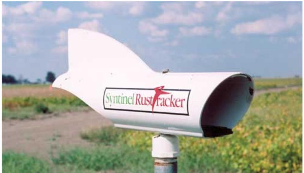
*Spore sampler used in the spore movement study. (John Rupe)*
