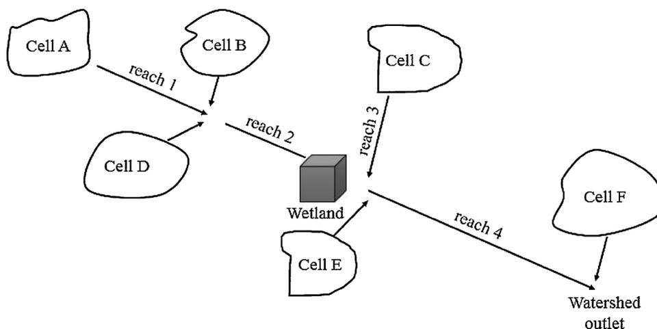
Fig. 2. Cell hydrology simulation in AnnAGNPS. For this simulation, the wetlands are located in the reach before the outlet to capture all the load generated by the watershed.
