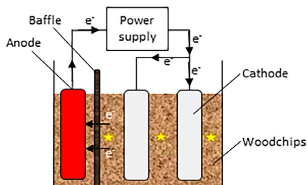
Fig. 1. Schematic of a batch bioreactor. The arrow indicates the direction of electron flow. The stars represent the sampling locations. A stainless-steel anode and two graphite cathodes were partially submerged in electrically stimulated woodchip bioreactors (BR1, BR2). The woodchip-only bioreactors (BR3, BR4) contained no anode or cathode.
