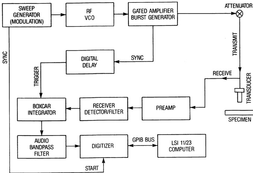
Figure 1. Swept Frequency Tone Burst Instrumentation.
