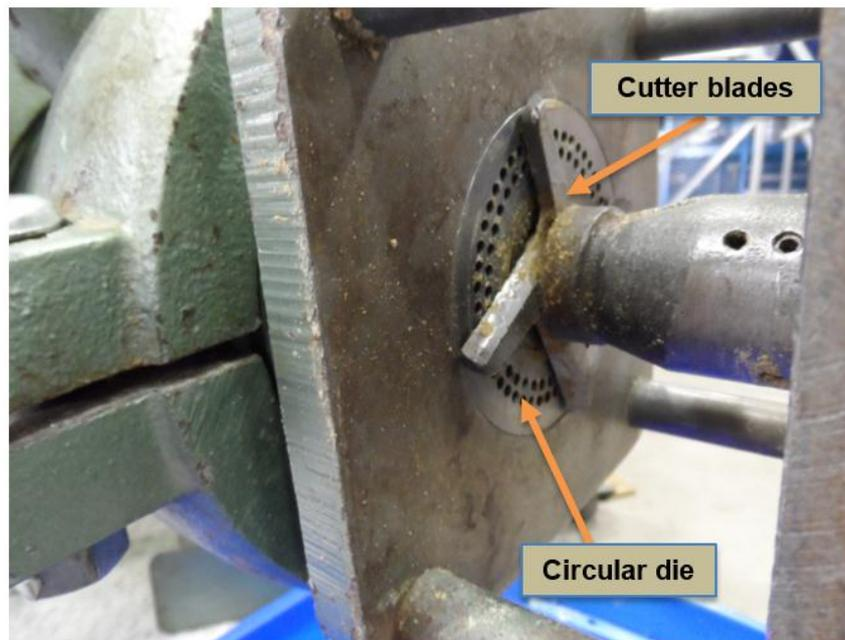
Figure 2. Example of a circular extruder die with multiple die openings
