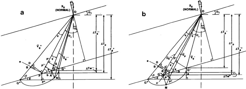
Fig. 3  $\bar{V}_w \times \bar{V}_p$  plane showing out of plane energy vectors. a) Points and angles used in Section III, the angles are:  $a = \pi - \theta_r$ ,  $b = \theta_i$ ,  $c = \pi - \psi - \theta_r$ ,  $d = \theta_i$ , and  $e = \psi$ . b) Additional angles used in Section IV are  $c' = \pi - \psi' - \theta_r$  and  $e' = \psi'$  (not shown).
