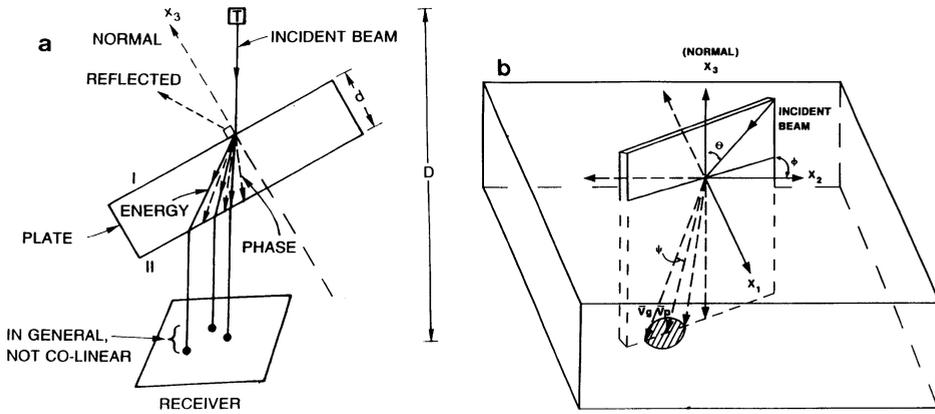
Fig. 1. a) Schematic diagram of the immersion system. b) "3-dimensional" diagram of the plate, refracted phase vector and cone of possible energy vectors (showing only one wave mode).
