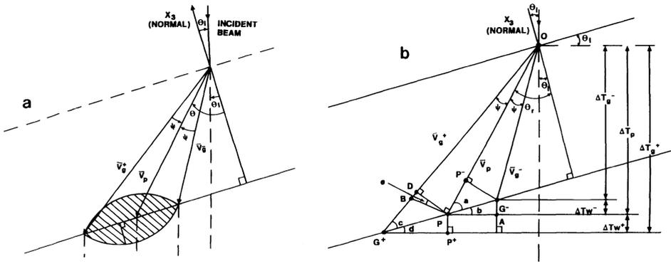
Fig. 2. a) A more detailed view of the  $\bar{V}_{wx}\bar{V}_p$  plane. b)  $\bar{V}_{wx}\bar{V}_p$  plane with points and angles used in Section I and II labelled. The angles are:  $a = \pi - \theta_r$ ,  $b = \theta_i$ ,  $c = \pi - \psi - \theta_r$ ,  $d = \theta_i$ , and  $e = \psi$ .
