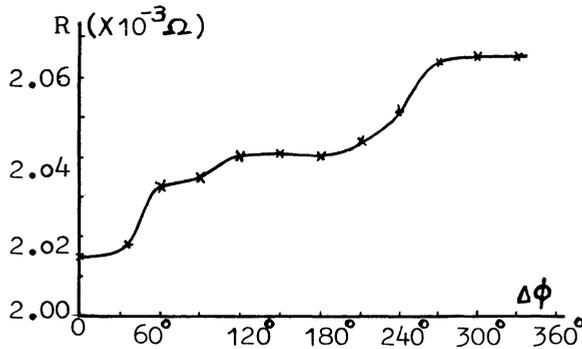
Fig. 4. The resistance  $R$  vs. twisting angle  $\Delta\phi$  of sample #2 which was plastically twisted at 120K. This curve is line 4 in Fig. 3.
