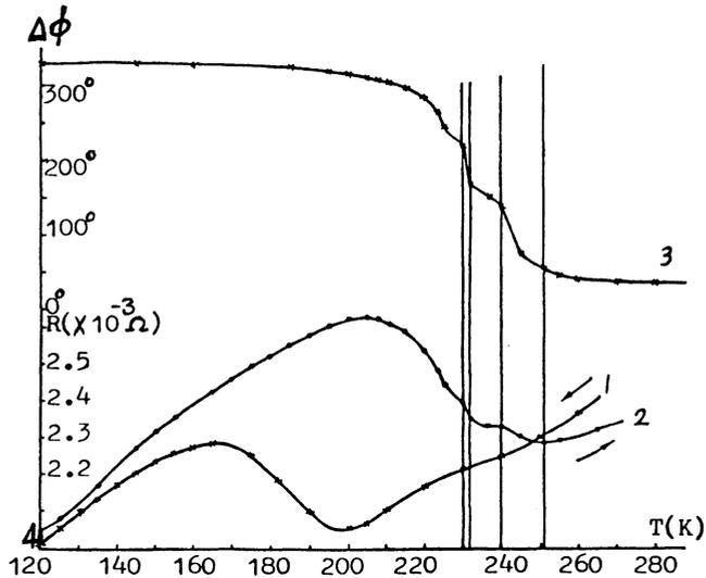
Fig. 3. The shape recovery and resistance change during SME in Cu-Zn sample #2 (Cu-40.2wt% Zn). Curve 1: The electric resistance  $R$  vs. temperature  $T$  on cooling; Curve 2: The  $R$ - $T$  curve on heating; Curve 3: The shape recovery on heating, the total recovering ratio is 92%; Curve 4: The sample was twisted plastically at constant temperature 120K which is below the  $M_f$
