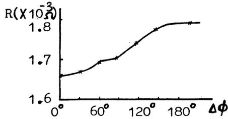
Fig. 2. The resistance  $R$  vs. twisting angle  $\Delta\phi$  of sample #1 which was plastically twisted at 135K ( $= M_S+7K$ ). This curve is line 4 in Fig. 1.
