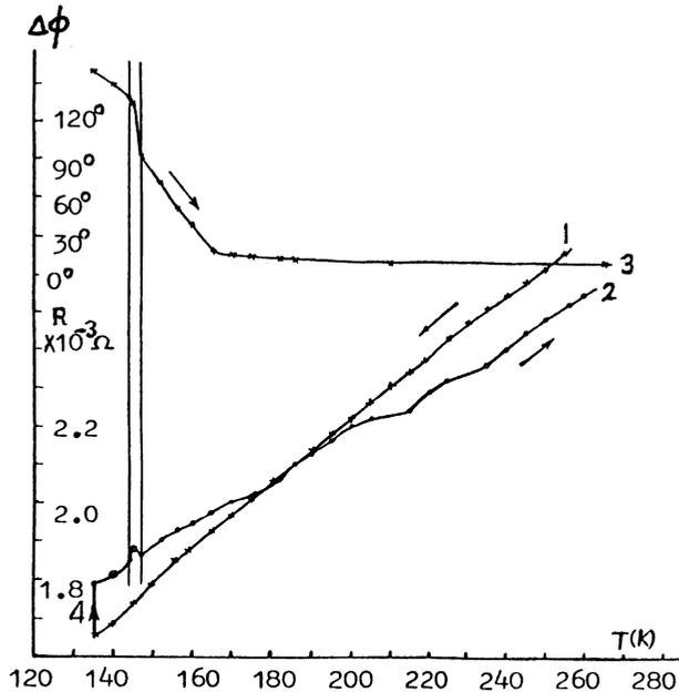
Fig. 1. The electric resistance change in Cu-Zn sample #1 (Cu-40.5wt% Zn) during SME above  $M_S$ . Curve 1: The resistance R vs. temperature T on cooling; Curve 2: The R-T curve on heating; Curve 3: The shape recovery on heating, the total recovering SME ratio is 94%; Curve 4: The sample was twisted plastically at constant temperature 135 K ( $=M_S + 7K$ ).
