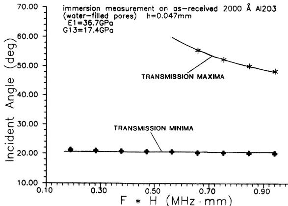
Fig. 6 The minimum- and maximum-transmission angles as functions of the product of frequency and sample thickness. The experimental data are shown as points. The best fitting curves, overlaid with the measured data, are obtained from the optimization of  $E_1$  to fit the minimum-transmission angles and subsequently of  $G_{13}$  to fit the maximum-transmission angles.
