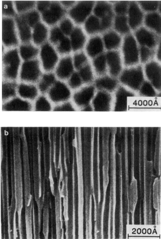
Fig. 3. Scanning electron microphotographs of the representative microstructure of the thin layer anodized  $\text{Al}_2\text{O}_3$ . (a) Top surface. (b) Cross section.
