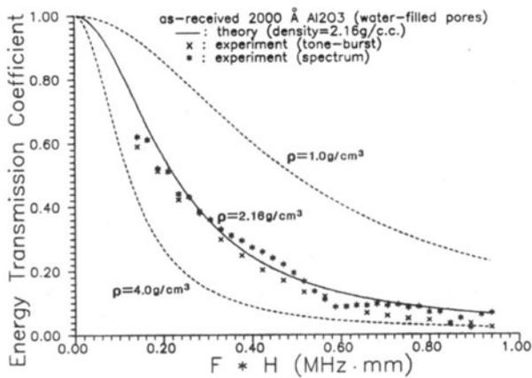
Fig. 4. Normal incident transmission coefficient and its dependence on the sample density. The discrete points are from experiment. The lines are calculated from theory [7] for different sample densities. The theoretical transmission coefficient corresponding to the measured sample density  $2.16 \text{ g/cm}^3$  is shown as the solid line. The calculated results are in good agreement with the measured data.
