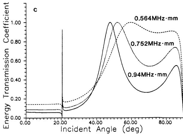
Fig. 1. Dependence of transmission coefficients on elastic constants and on the product of frequency and sample thickness. (a) Effect of in-plane Young's modulus,  $E_1$ . (b) Effect of interlayer shear modulus,  $G_{13}$ . (c) Effect of frequency and sample thickness.
