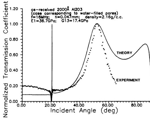
Fig. 5 The measured and calculated transmission coefficients as a function of incident angle. The measured data are shown as discrete points. These data are overlaid on the theoretical transmission coefficients calculated by using the reconstructed elastic constants  $E_1$  and  $G_{13}$ . The other elastic moduli needed for calculation are taken from Nielsen's model (see Table 1).
