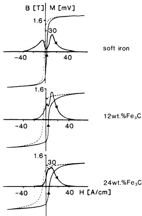
Fig. 1. Magnetic Barkhausen noise-hysteresis curves. Microstructure state: perlitic globular
