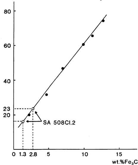
Fig. 5. Normalized amplitude  $M^*$  of magnetic Barkhausen noise as a function of cementite content
