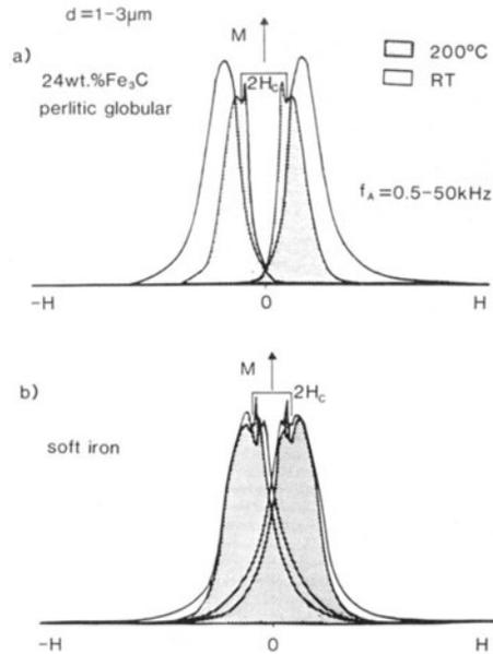
Fig. 4. Magnetic Barkhausen noise for perlitic state (a) and soft iron (b) at 200°C and room temperature
