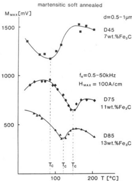
Fig. 3. Maximum of Barkhausen noise amplitude as a function of temperature
