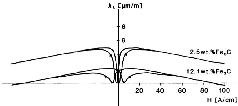
Fig. 2. Longitudinal Magnetostriction
