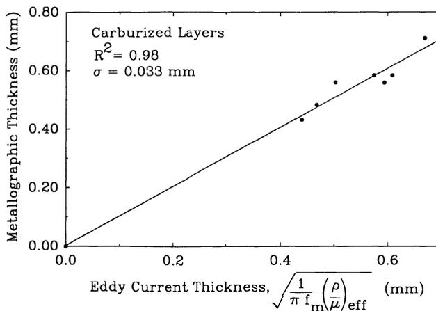
Figure 2. Correlation between the thickness of the surface layer measured using optical techniques and the eddy current thickness defined as  $\delta_{\text{eff}}$  for  $H_c = H_{c_{\text{max}}}$ , the maximum value of , coercivity.
