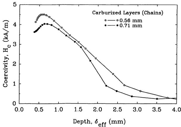
Figure 1. Experimental coercivity profiles as a function of the effective penetration depth,  $\delta_{\text{eff}}$  for two chain samples with surface layer thicknesses of 0.56 and 0.71 mm. The value of  $\rho/\mu$  corresponding to the solid line (best fit) is  $(\rho/\mu)_{\text{eff}} = 2.08 \times 10^{-8} \Omega\text{-m}$ .
