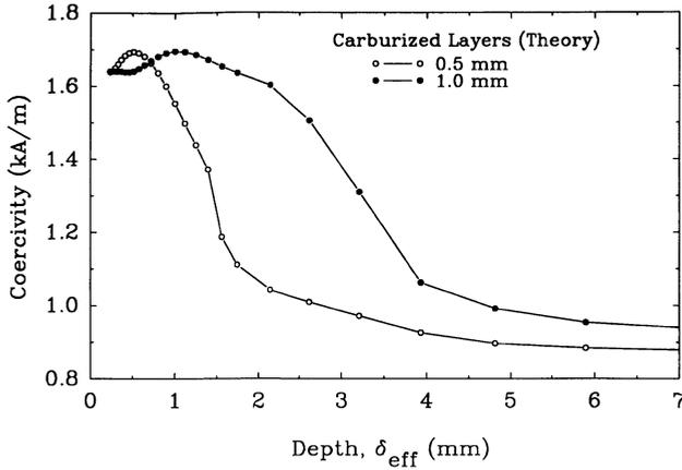
Figure 4. The calculated coercivity profiles as a function of the effective penetration depth for cylinders with surface layers of 0.5 and 1.0 mm thick. The resistivity,  $\rho = 2.0 \times 10^{-7} \Omega\text{-m}$ , and incremental permeability of 38.36 was used to calculate  $\delta_{eff}$ . Note that the general shape of the curves is in good agreement with figure 1.
