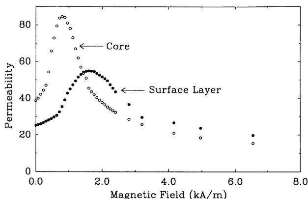
Figure 3. The variation of the relative incremental permeability as a function of the applied magnetic field for the core and surface layers of a cylinder used in the calculation of the impedance curves.
