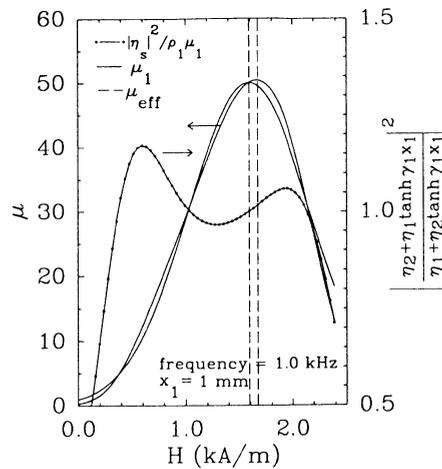
Figure 5. The variation of  $\mu_{\text{eff}}$ ,  $\mu_1$ , and the squared term in equation (11) of the text as a function of the magnetic field. This figure shows how the measured values of coercivity can be shifted to values higher than  $H_{c \text{ surf}}$
